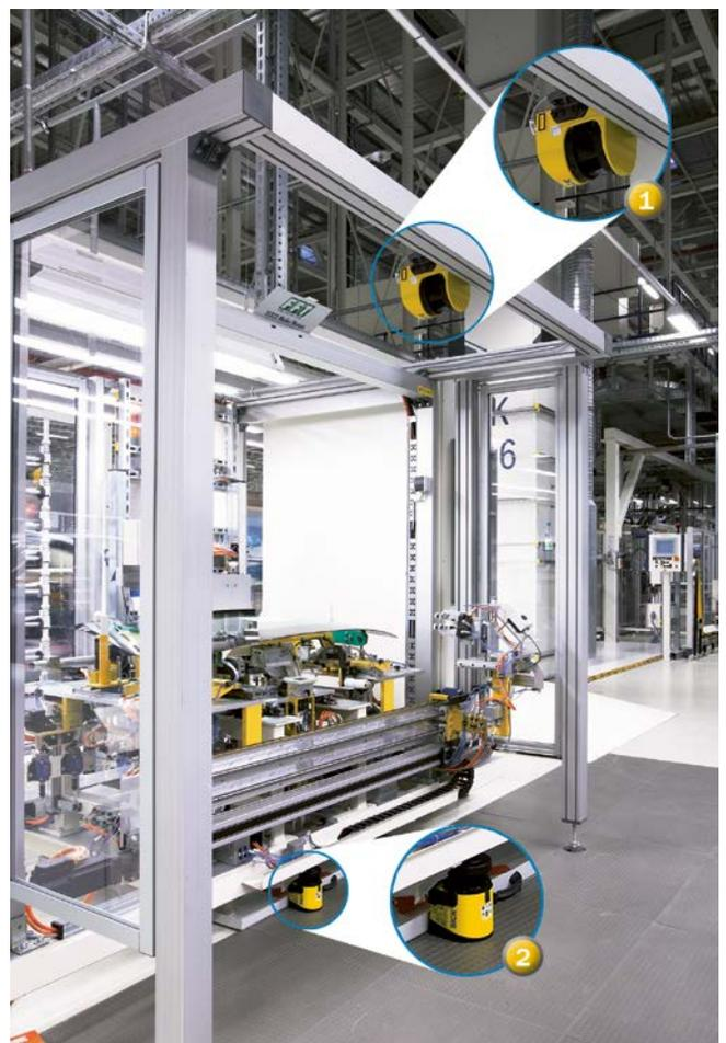
Safety laser scanner on a machining center as safety function pos. 1, initiating a stop and safety function pos. 2, preventing unexpected start
