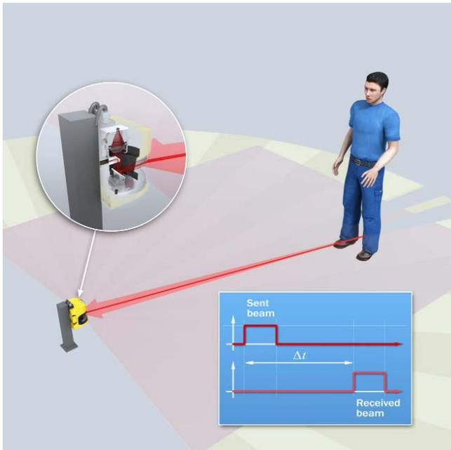
Fig. 10: The safety laser scanner forms a protective field. The object is detected by reflection and time-of-flight measurement of the transmitted laser beam.
