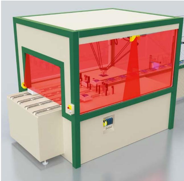
Fig. 12: Hazardous point protection using a safety camera system on a handling robot in solar cell production.
