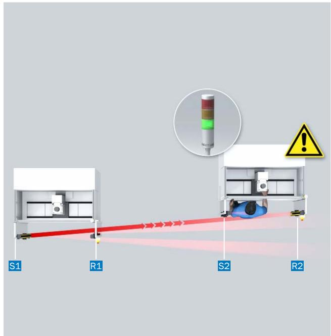
Fig. 19: By mutual interference the ESPE protection is rendered inoperative.
