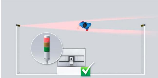
Fig. 15: The person is detected reliably and the hazardous movement stopped.
