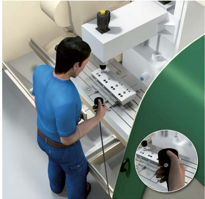
The machine start shall not be initiated solely by the actuation of an enabling device. Instead, movement is only permitted as long as the enabling device is actuated.
