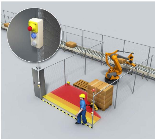
Fig. 8: Stationary hazardous area protection with a safety laser scanner.
