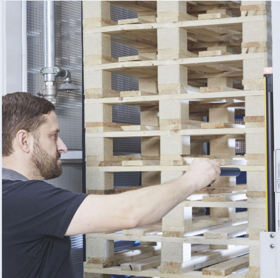
Initial inspection of the opto-electronic protective devices before the machine is put into operation for the first time verifies the proper mounting and correct functioning of the protective devices for the detection of persons and documents this in accordance with the obligation to provide evidence.
