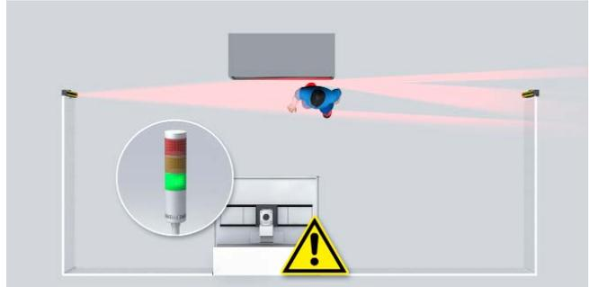
Fig. 16: Reflection hinders the protective effect of the ESPE is nullified.
