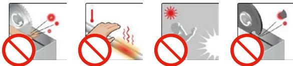
Fig. 2: Typical hazards where electro-sensitive protective cannot be used.
