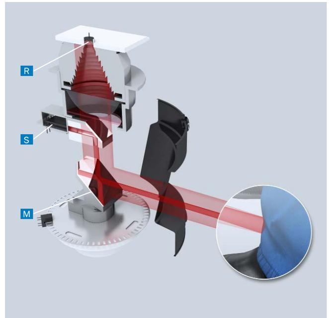
Fig. 11: Basic structure of a laser scanner.
