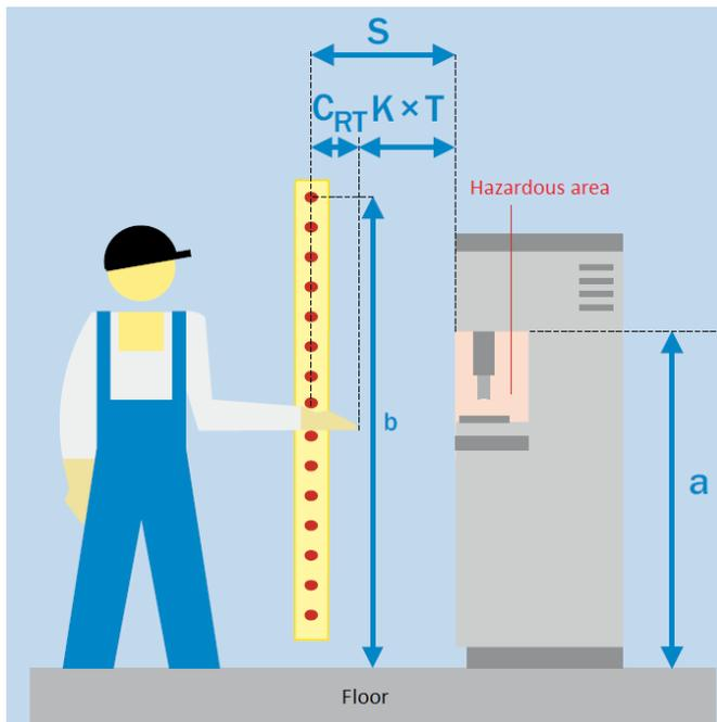
Fig. 14: Parameters for determining the required minimum distance or protective field height when approaching at a right-angle.
