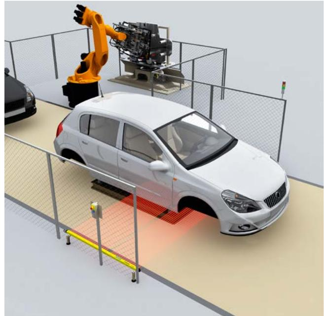
Fig. 21 and 22: Entry/exit function with horizontally arranged safety light curtain in a processing station of an automobile assembly line.
