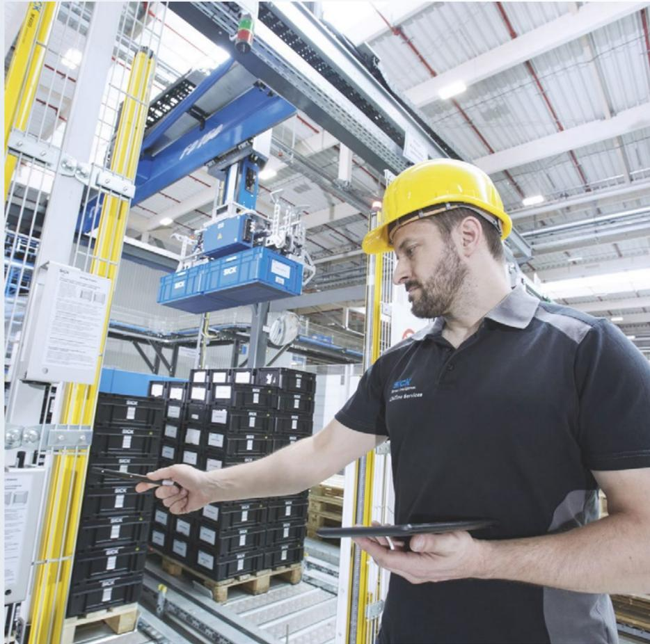
During periodic inspections, the effectiveness of the protective devices is checked and documented. This is done taking into account the current use of the machine within the legally required inspection intervals.
