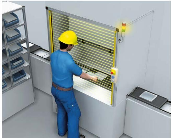
Single break PSDI mode on an automatic assembly system with safety light curtain. During loading, the tool is at the top point. After the operator leaves the protective field, the assembly process gets underway.
