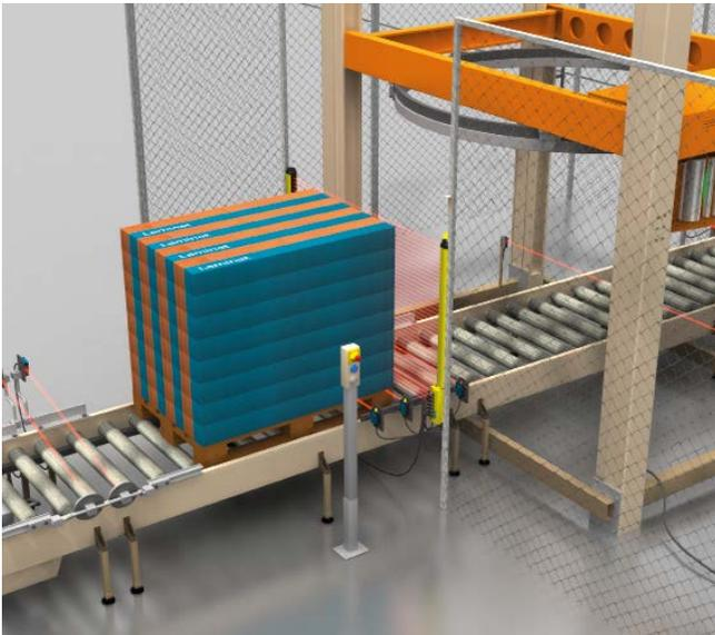
Fig. 20: Muting function with safety light curtain and muting sensors on a wrapping machine.
