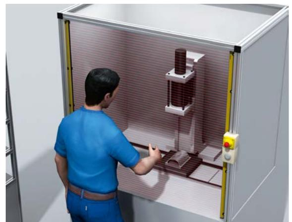
Fig. 6: Hazardous point protection using a safety light curtain.
