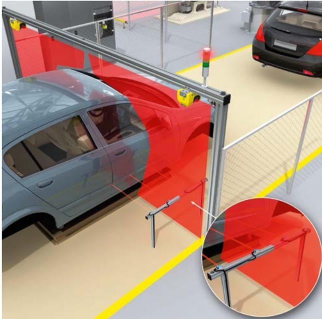
Fig. 23: Passing of material with safety laser scanners, horizontal protective fields and adequately positioned sensors
