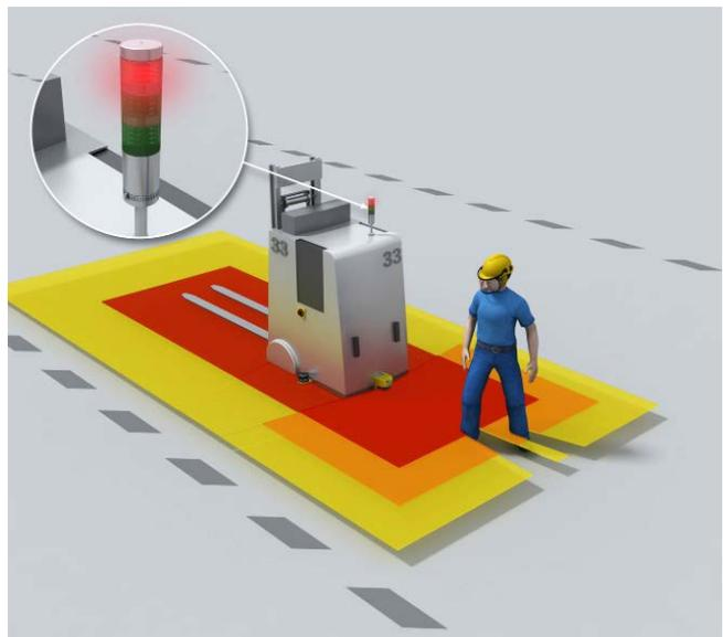
Fig. 9: Mobile hazardous area protection with a safety laser scanner.
