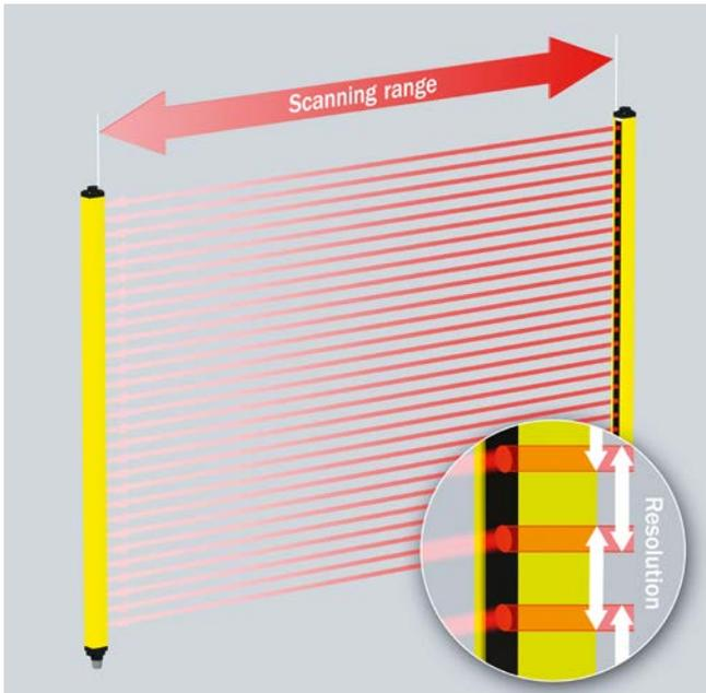
Fig. 7: Typical structure of a safety light curtain with sender and receiver.
