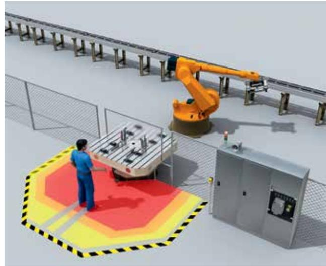
**Mobile hazard area protection: Detection of a person approaching the hazard area**
