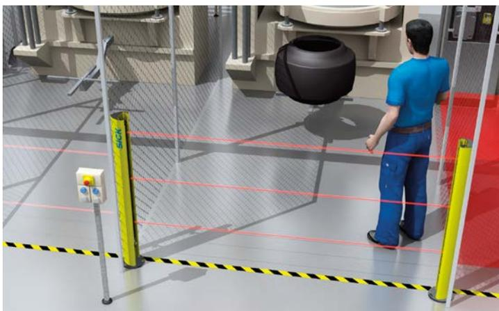
Fig. 5: Access protection using a multiple light beam safety device.
