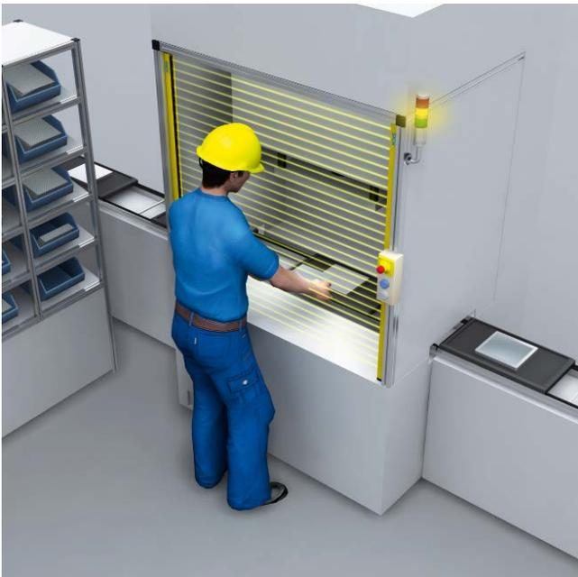
Fig. 26: Single break PSDI mode on a press with safety light curtain. During the work piece loading, the press die (ram) is at the top point. After release of the protective field by the operator, the die automatically moves downward.
