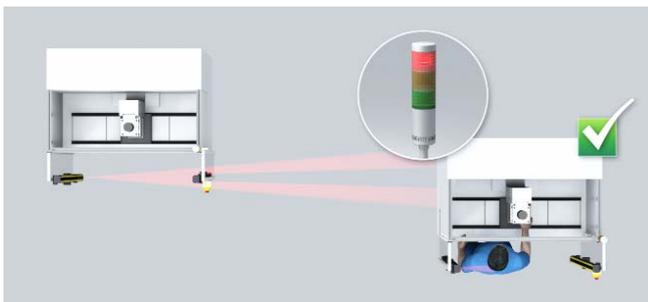
Fig. 17 and 18: There is no mutual interference between protective devices. The person is detected reliably by encoding the beams or by arranging the protective adequately.
