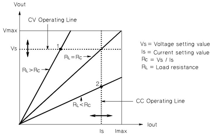
**Figure 7-5. Output Characteristics**
