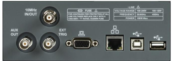
Connectivity includes External Trigger Input, Pass/Fail and Trigger Out, USB Device (USB TMC) and LAN for remote control, and a Kensington Lock security point.
