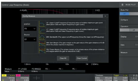
The measurement screen enables the setting of five common measurements: Upper cutoff, lower cutoff frequency, bandwidth, gain margin and phase margin, in addition there are user settable measurement cursors.
