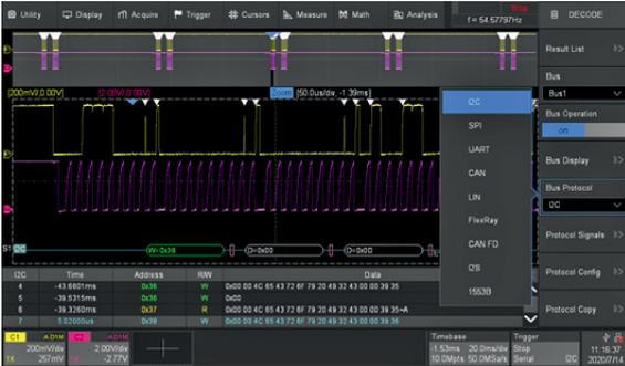
Trigger and decode up to 2 common embedded and automotive serial buses, I<sup>2</sup>C, SPI, UART, LIN, CAN, CAN FD, FlexRay, I<sup>2</sup>S, MIL-STD-1553B, SENT and Manchester. Protocol information can be quickly and intuitively displayed, time aligned with the waveform and in table format.
