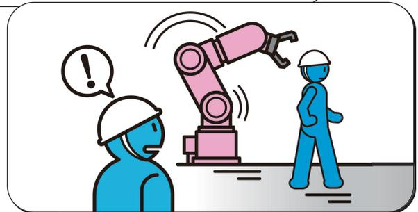
Machinery hazards occur in the areas, where the human workspace overlaps the machine workspace. Preventing machinery hazards begins by eliminating mechanisms that facilitate hazardous conditions. The following principles can be used to achieve this goal.
