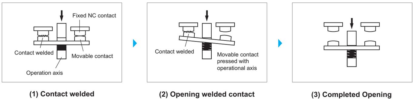
Contacts with direct opening action can be opened by applying the specified direct operating force (DOF) to the actuator to move it to the end of the direct operating travel (DOT) even when the force equivalent to the contact welding force (10 N) is applied in the direction of closing the contacts. The gap between open contacts must withstand the specified impulse voltage.
