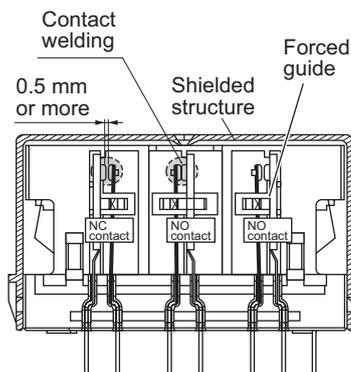
(a) When contact welding occurs in the NO contact
