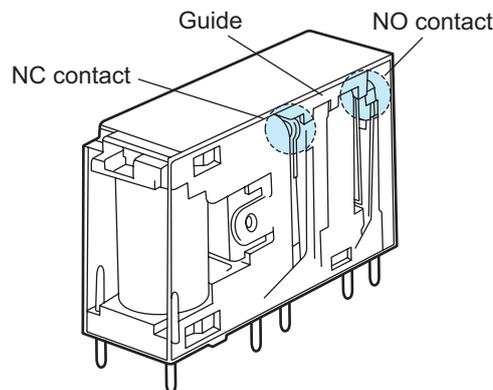
• Structural Comparison of General Relays and Relays with Forcibly Guided Contacts
