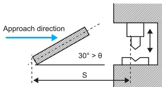
When the angle of the detection area is less than  $\pm 30^\circ$  with respect to the approach direction, the approach is considered as parallel approach and the calculation formula of B is applied.
