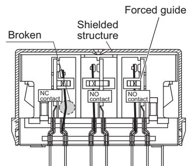
• The above shielded structure protects other contacts from being affected by the failure.
