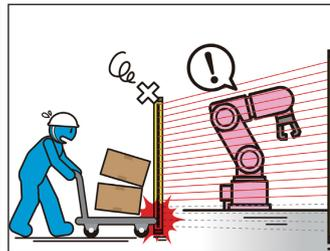
The machine stops safely even if a failure occurs on light curtains.
