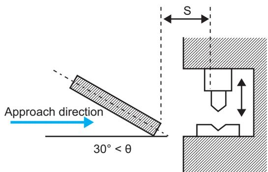
When the angle of the detection area exceeds  $\pm 30^\circ$  with respect to the approach direction, the approach is considered as vertical approach and the calculation formula of A is applied.
