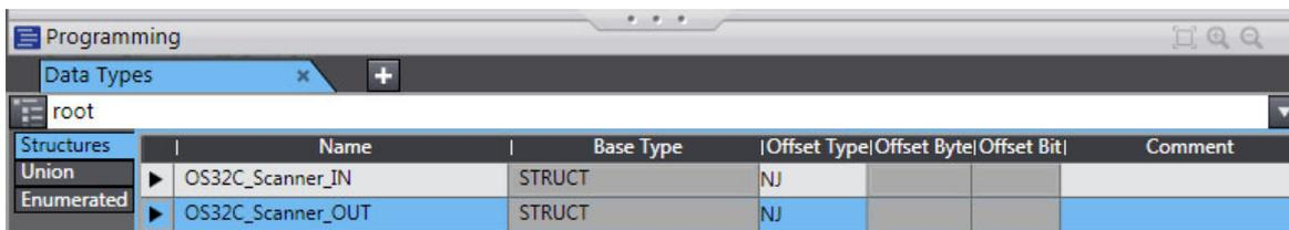
Fig. 7-5 OS32C IN and OUT Structure Data Types
