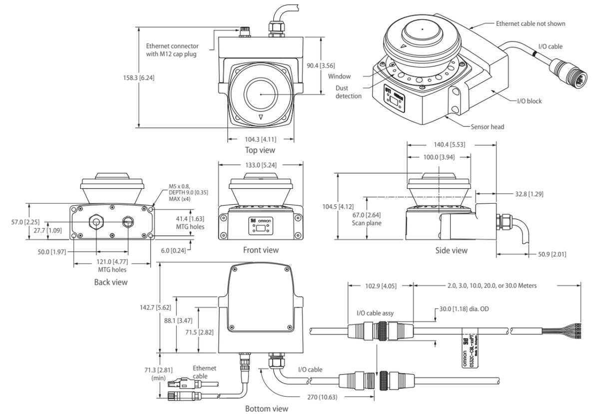
OS32C with side location cable entry - OS32C-SP1/OS32C-SP1-DM
