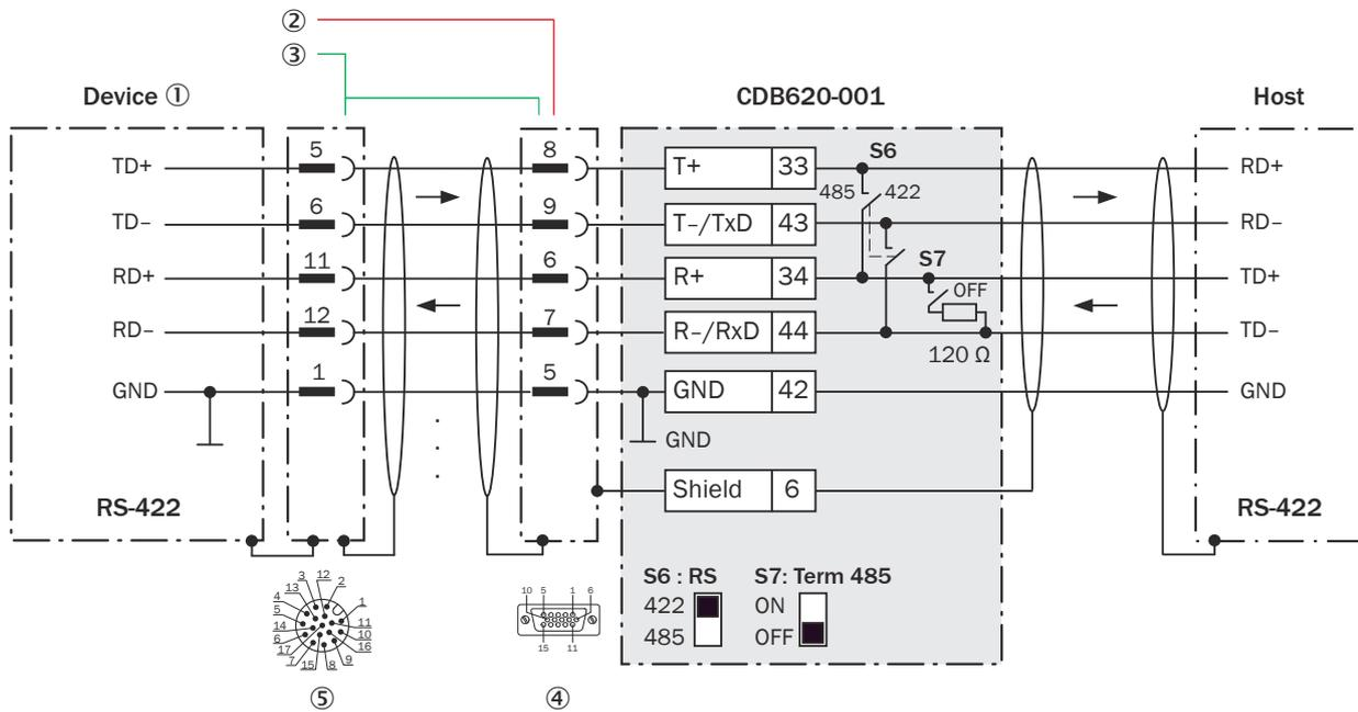
Figure 157: Wiring data interface RS-422 of the device in the CDB620-001 connection module, Ethernet variant with male connector, M12, 17-pin, A-coded
