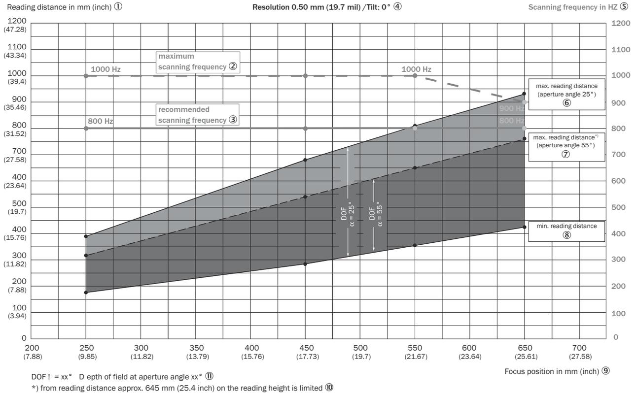
Depth of field ranges of the CLV651 line scanner with front reading window: Resolution 0.5 mm (19.7 mil); inclination angle 0°; aperture angle 25°/55°
