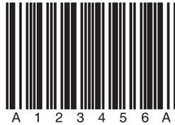
Fig. 2-2: Codabar example
