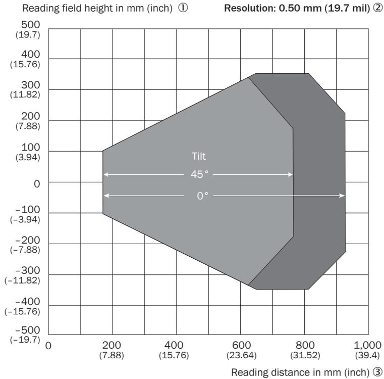
Figure 130: Reading field diagram for CLV651-Xxx0, low density, line ( $X = 0$ ), glass viewing window, at the front, tilt angle  $45^\circ$  and  $0^\circ$
