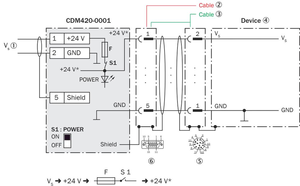
Figure 184: Connecting supply voltage for the device in the CDM420-0001 connection module, Ethernet variant with male connector, M12, 12-pin, A-coded
