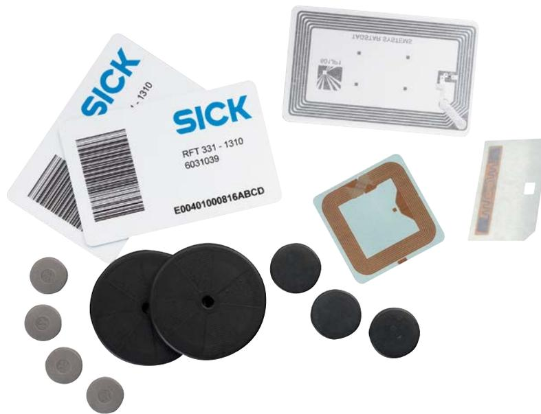
Figure 2: Passive HF and UHF RFID transponders in various forms facilitate the attachment to objects and the use as identification cards. The antenna and chip designs of UHF and HF tags differ considerably due to the different ways that the energy and data transmission work (tag on the far right: UHF, the rest: HF).
