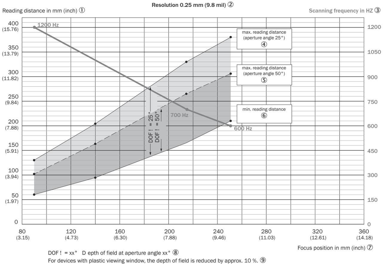
Figure 108: Depth of field ranges for CLV640-Xxx0, line (X = 0) or raster (X = 1), 0.25 mm resolution, glass viewing window, at the front. Minimum and maximum reading distance as a function of focus position and aperture angle
