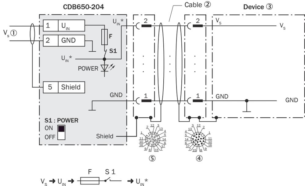
Figure 171: Connecting supply voltage for the device in CDB650-204 connection module.
