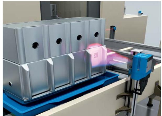
Figure 8: Matrix cameras read printed or directly marked 1D and 2D codes, for example during the package sorting process (left) or for unique identification of parts such as motor blocks during production (right).
