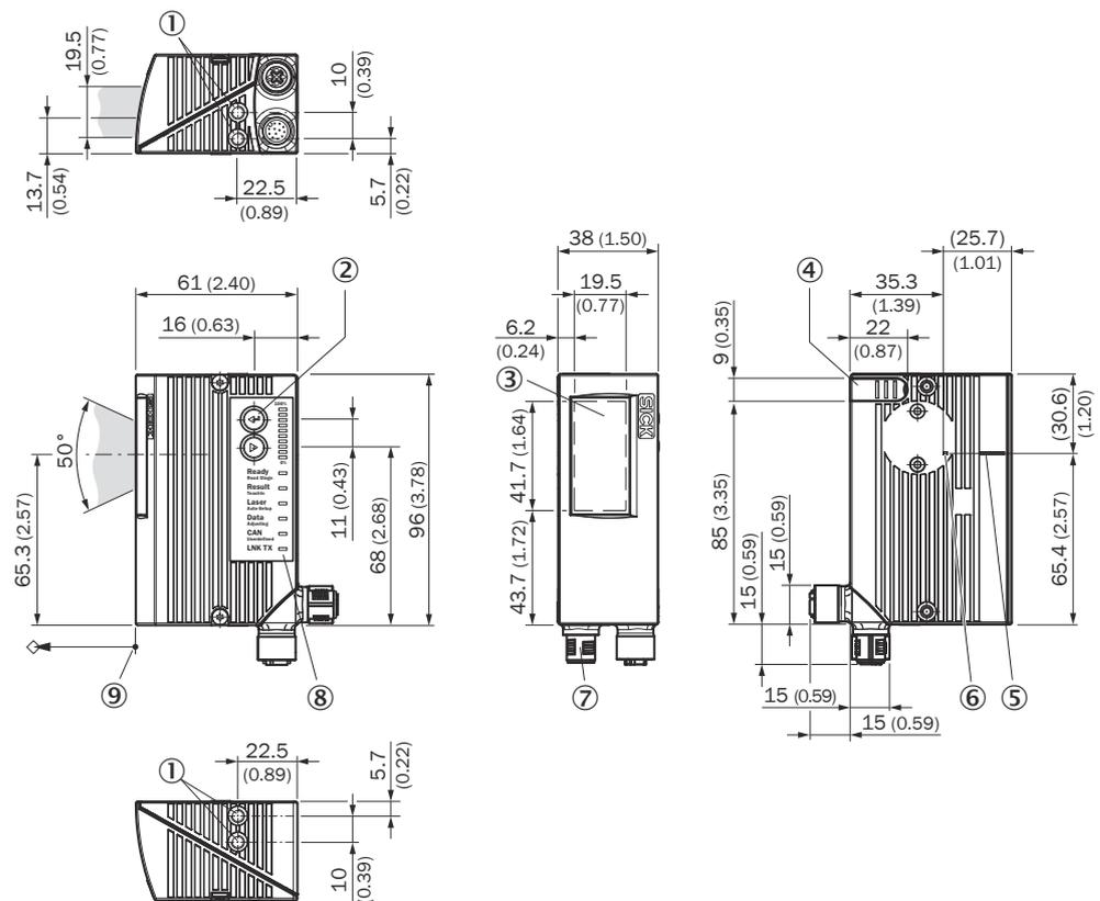
Figure 67: CLV63x to CLV65x: Ethernet variant in standard housing, with front viewing window and swivel connector. structure and device dimensions, unit: mm (inch), decimal separator: period
