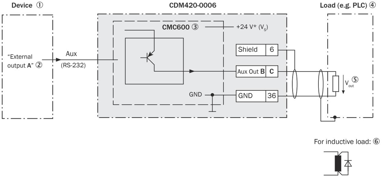
Figure 219: Wiring “Aux Out 1” and “Aux Out 2” external digital outputs of the device in the connection module CDM420-0006.
