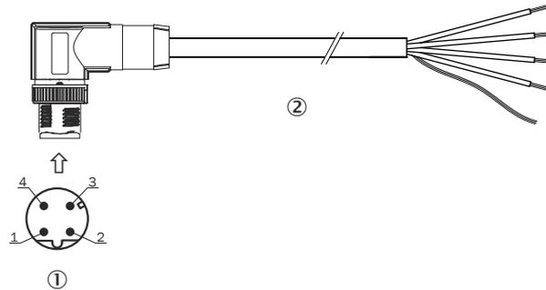
Figure 66: Adapter cable, e.g. part no. 2106174 (2 m)
