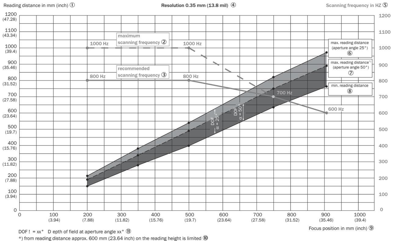
Depth of field ranges of the CLV650 line scanner with oscillating mirror: Resolution 0.35 mm (13.8 mil)
