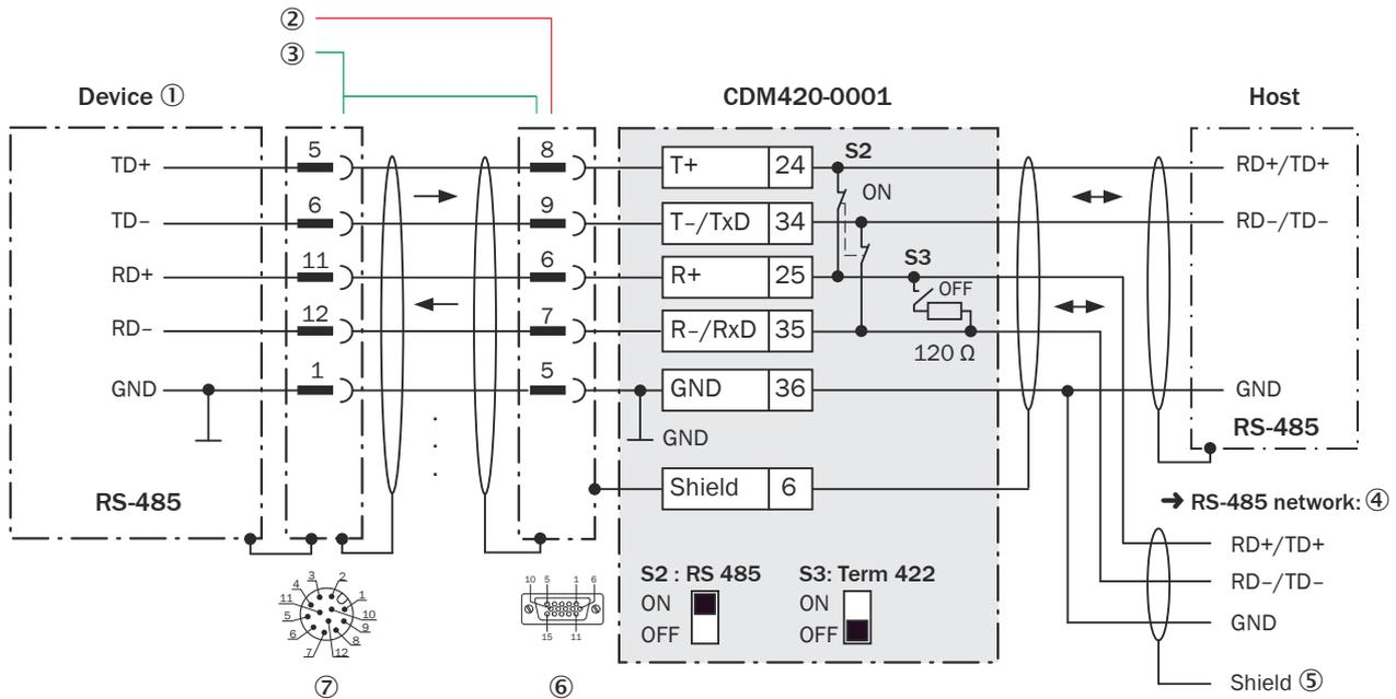
Figure 190: Wiring data interface RS-485 of the device in the CDM420-0001 connection module, Ethernet variant with male connector, M12, 12-pin, A-coded
