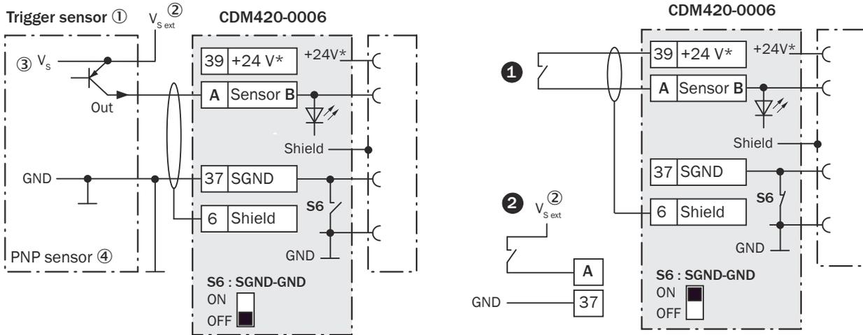
Figure 214: Left: Trigger sensor connected potential-free and supplied with power externally. Right: alternative switch, ① supplied with power by connection module CDM420-0006 or ② connected volt-free and supplied with power externally. Now select switch setting S6 as shown in the left figure.
