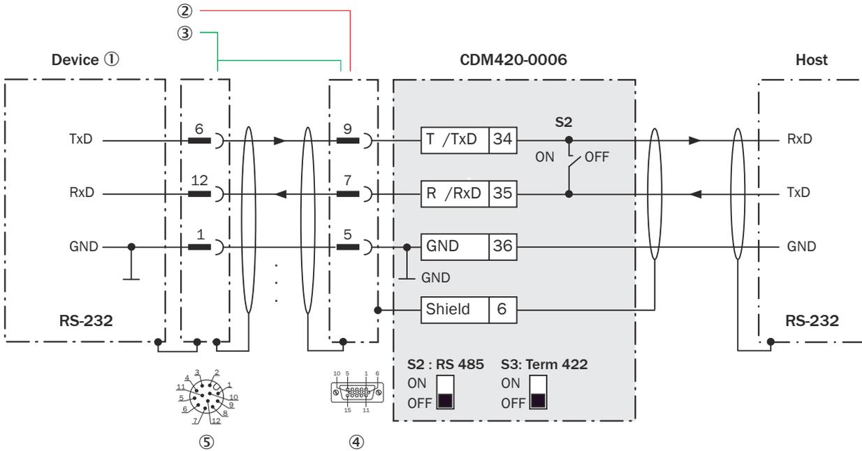
Figure 205: Wiring data interface RS-232 of the device in the CDM420-0006 connection module, Ethernet variant with male connector, M12, 12-pin, A-coded
