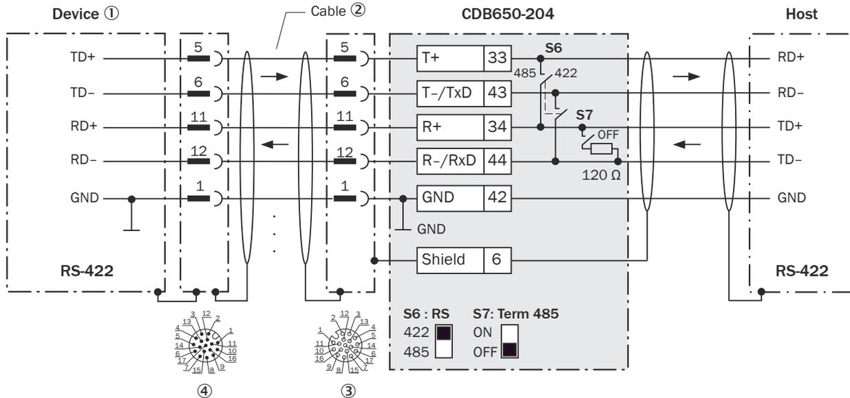
Figure 173: Wiring data interface RS-422 of the device in the connection module CDB650-204
