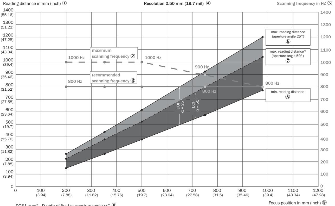
Depth of field ranges of the CLV650 line scanner with front reading window: Resolution 0.50 mm (19.7 mil)
