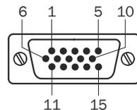
Figure 45: Male connector, D-Sub-HD, 15-pin
