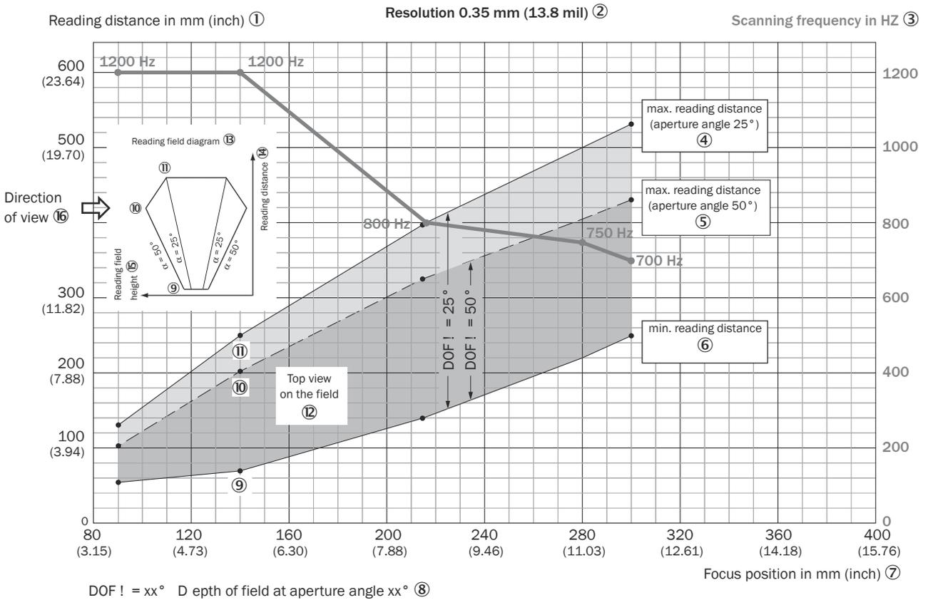
Figure 106: Meaning of the marks ⑨, ⑩ and ⑪ in the reading field diagram ⑬ in relation to the depth of field diagram
