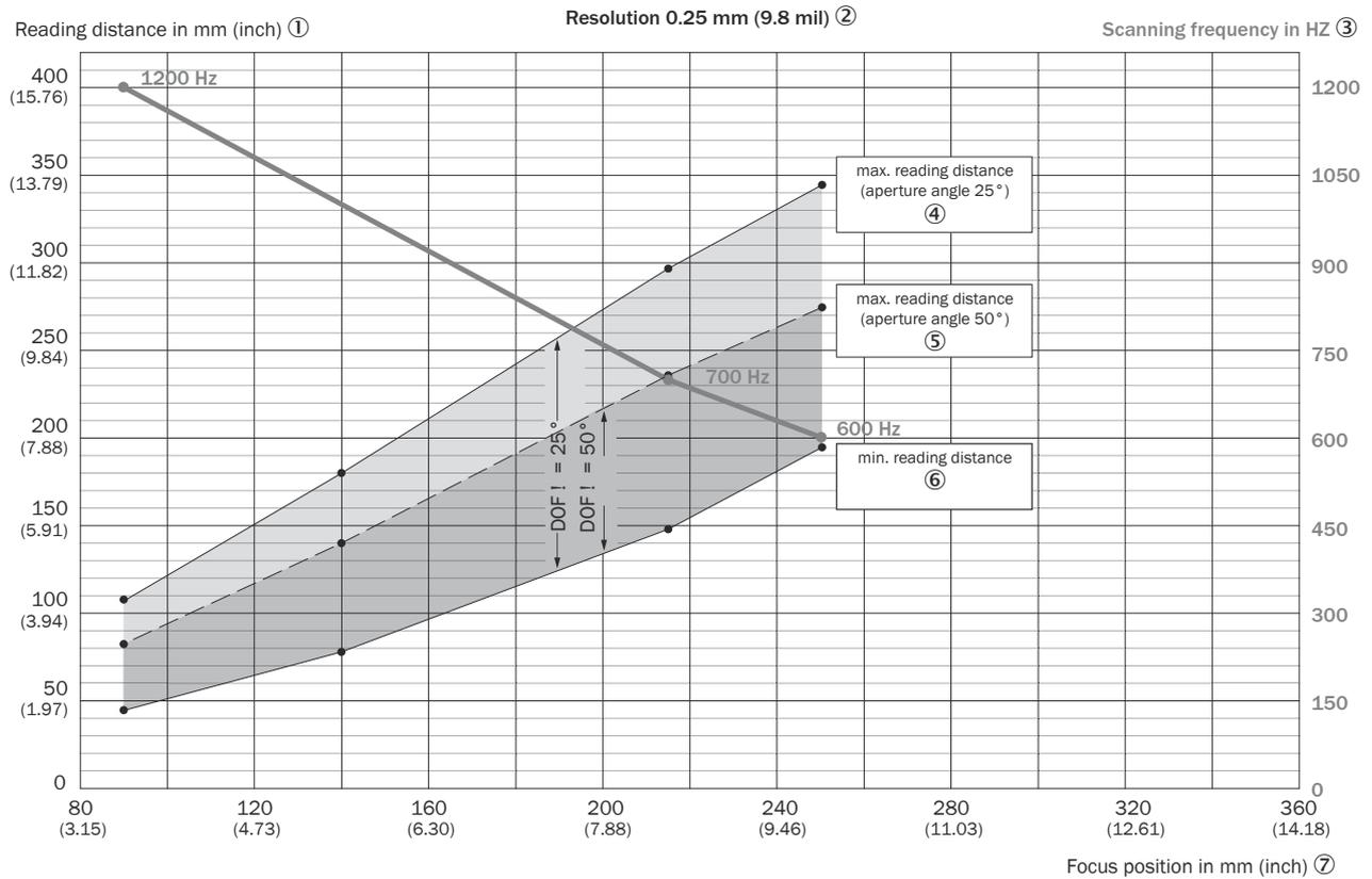
Figure 113: Depth of field ranges for CLV640-Xxx0, line (X = 2) or raster (X = 3), 0.25 mm resolution, glass viewing window, on the side. Minimum and maximum reading distance as a function of focus position and aperture angle
