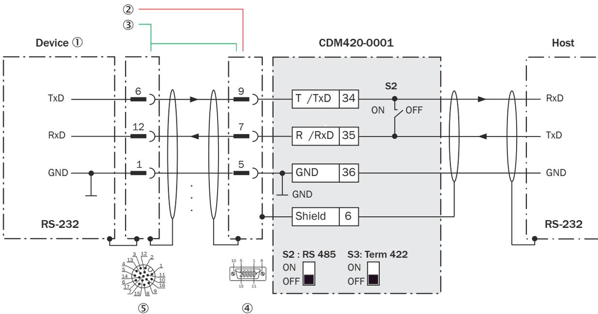
Figure 187: Wiring data interface RS-232 of the device in the CDM420-0001 connection module, Ethernet variant with male connector, M12, 17-pin, A-coded
