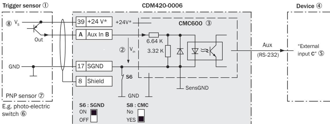
Figure 215: Trigger sensor supplied with power by connection module CDM420-0006.
