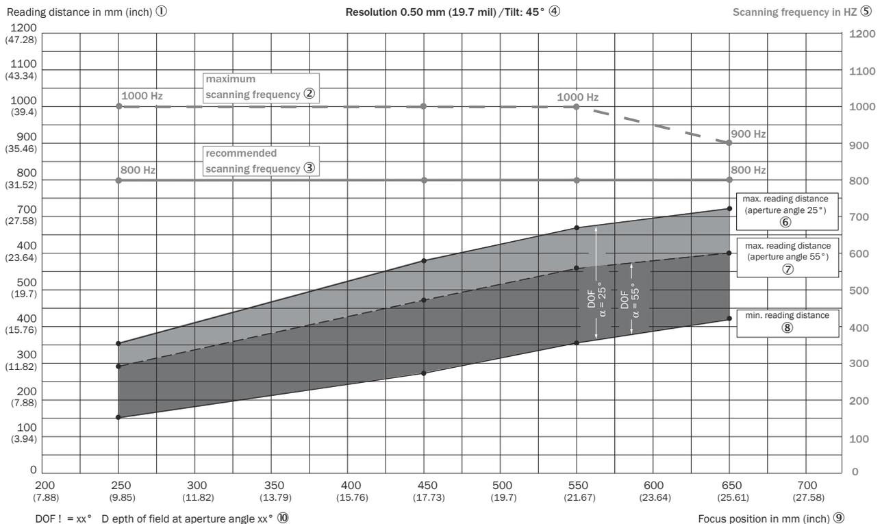
Figure 145: Depth of field ranges of the CLV651-6xx0, 0.50 mm resolution, line with oscillating mirror, glass viewing window, on the side. Minimum and maximum reading distance as a function of the focus position and aperture angle. Tilt angle 45°, aperture angle 25° or 55°
