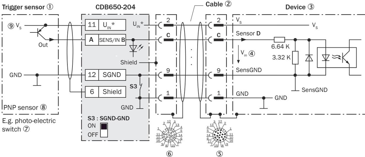
Figure 176: Trigger sensor supplied with power by connection module CDB650-204
