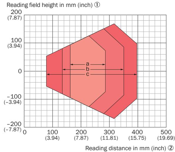
Figure 90: Reading field diagram for CLV631-6xx0, mid range, line scanner with oscillating mirror, glass viewing window, on the side
