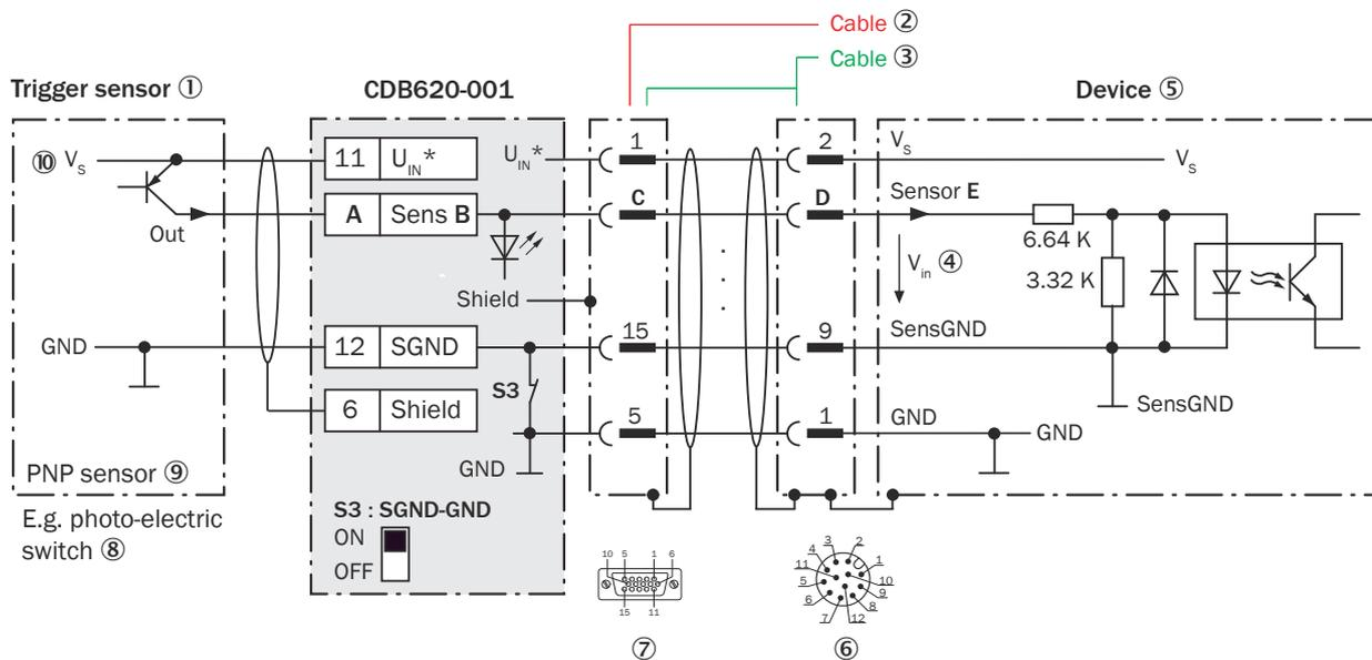
Figure 161: Trigger sensor supplied with power by connection module CDB620-001, Ethernet variant with male connector, M12, 12-pin, A-coded
