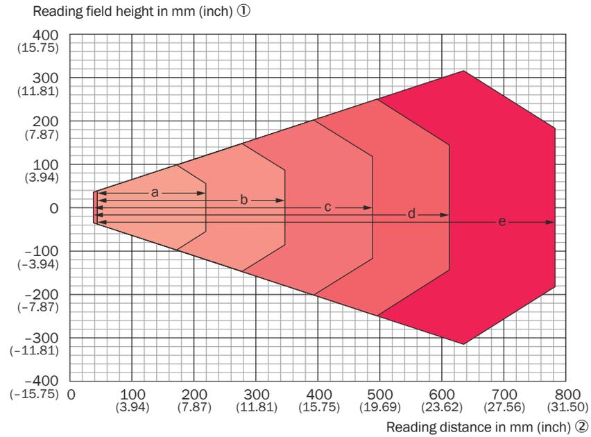
For devices with plastic reading window (CLV640-3000S01):
