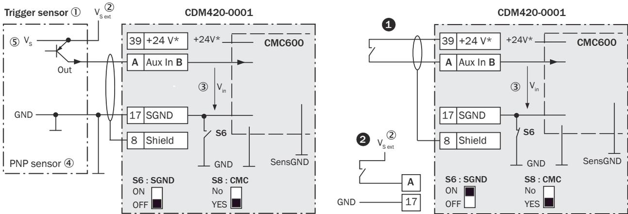
Figure 197: Left: Trigger sensor connected potential-free and supplied with power externally. Right: Alternatively switch, ❶ supplied with power by connection module CDM420-0001 or ❷ connected potential-free and supplied with power externally. Switch setting S3 then as in left figure.
