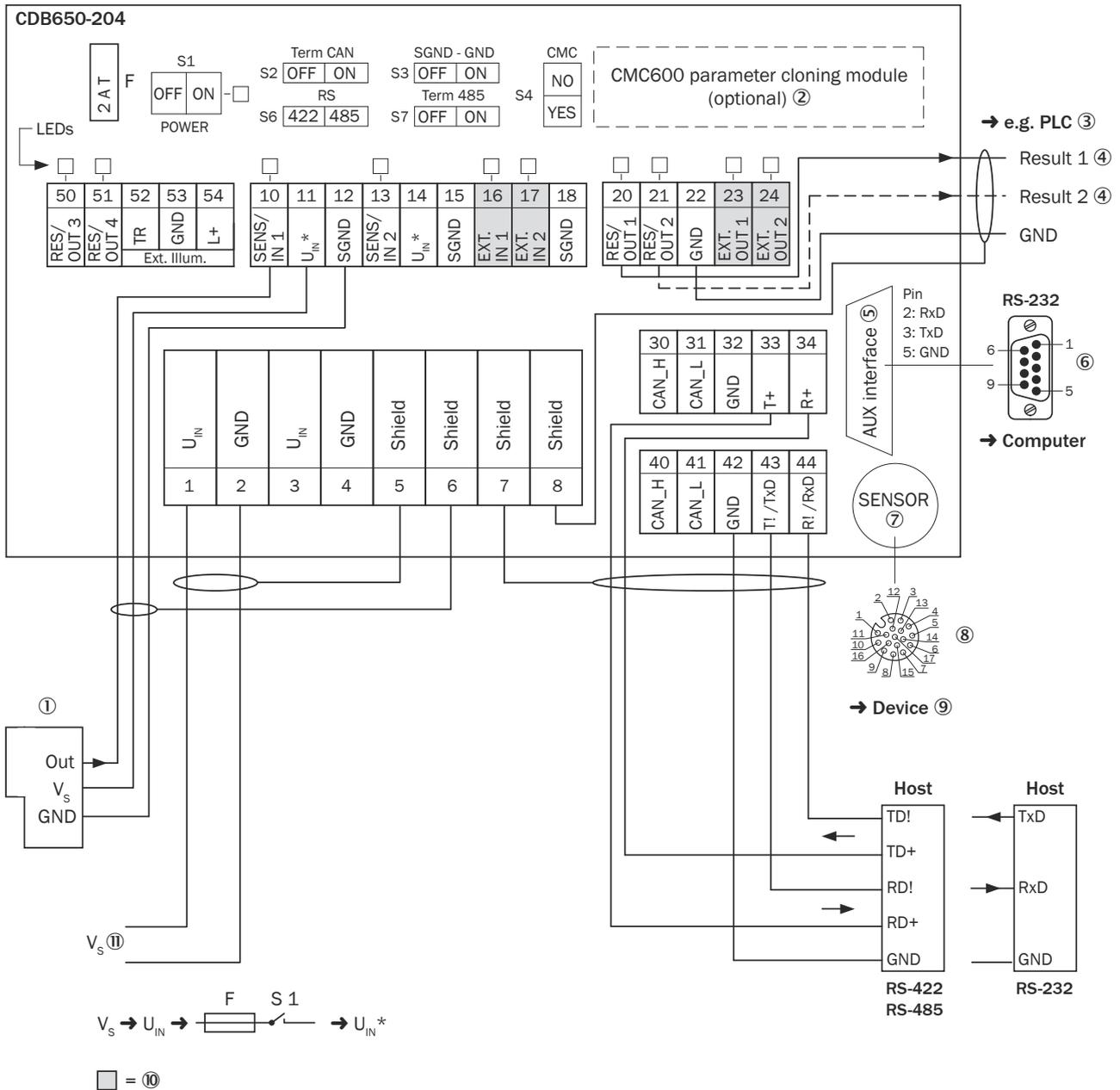
Figure 170: Overview: connection of device and peripherals to the CDB650-204 connection module
