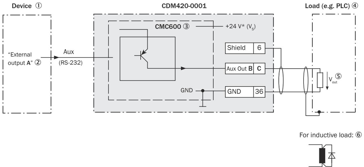
Figure 200: Wiring external digital outputs “Aux Out 1” and “Aux Out 2” of the device in the connection module CDM420-0001.
