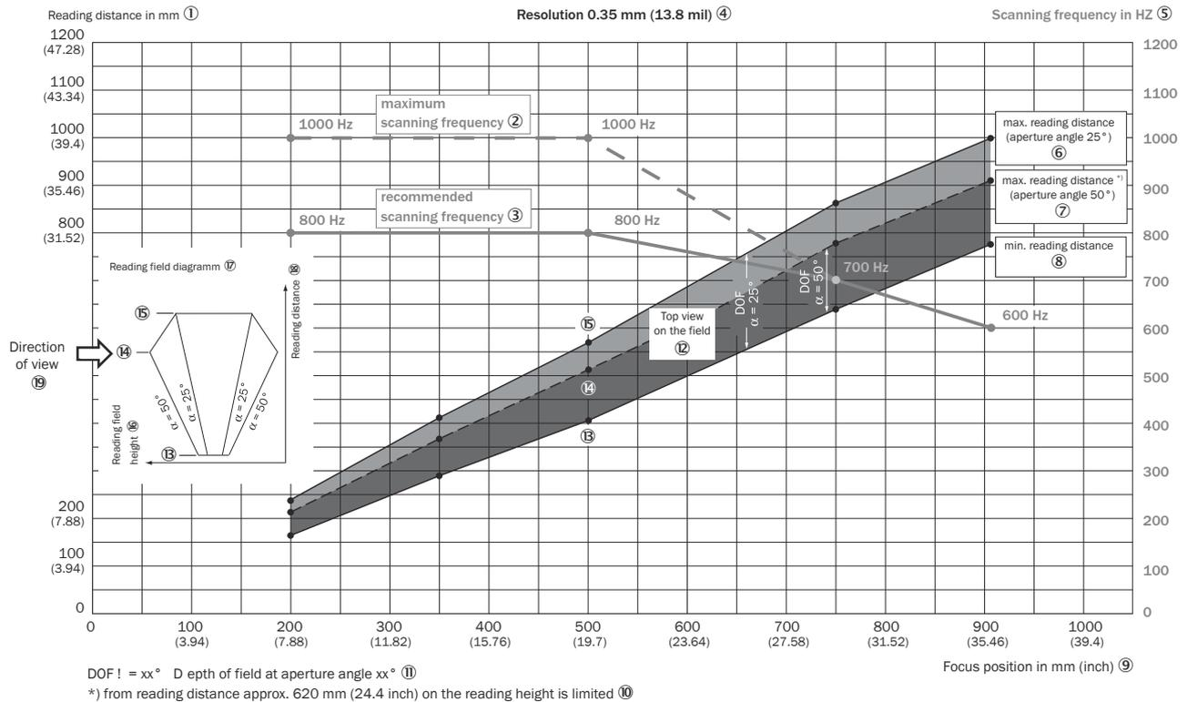
Figure 133: Meaning of the marks ⑬, ⑭ and ⑮ in the reading field diagram ⑭ in relation to the depth of field diagram
