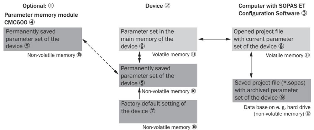
Figure 55: Configuration with SOPAS ET and saving the parameter set
