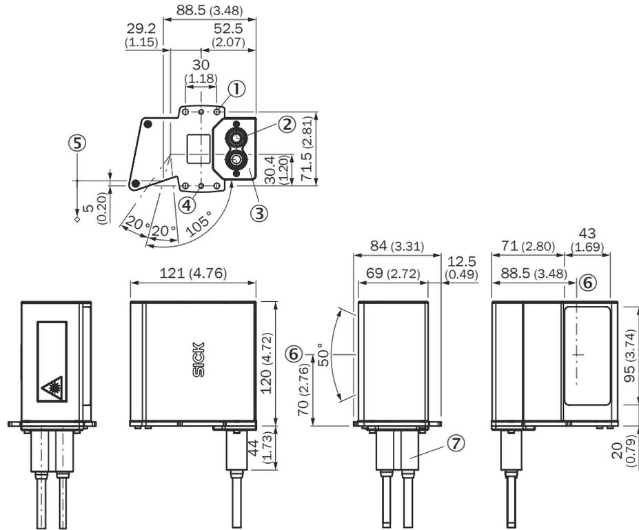
Figure 13: CLV63x/CLV64x: Ethernet variant in IP69K protective housing, with oscillating mirror (side viewing window) and two M12 connections. structure and device dimensions, unit: mm (inch), decimal separator: period
