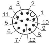
Figure 43: Male connector, M12, 12-pin, A-coded
