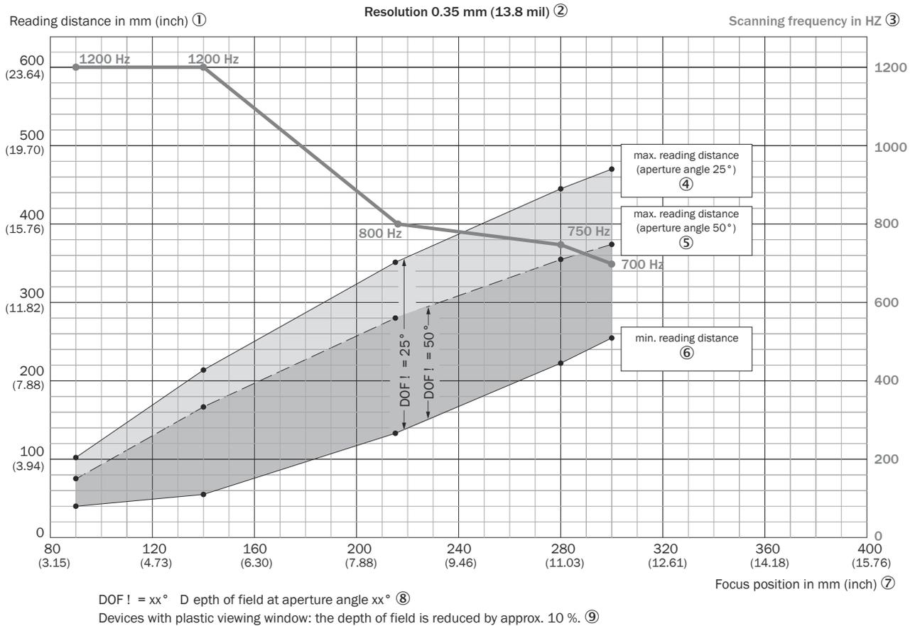
Figure 119: Depth of field ranges for CLV640-6xx0, 0.35 mm resolution, oscillating mirror, glass viewing window, on the side. Minimum and maximum reading distance as a function of focus position and aperture angle
