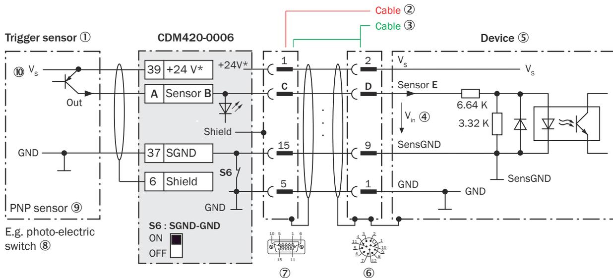
Figure 212: Trigger sensor supplied with power by connection module CDM420-0006, Ethernet variant with male connector, M12, 12-pin, A-coded
