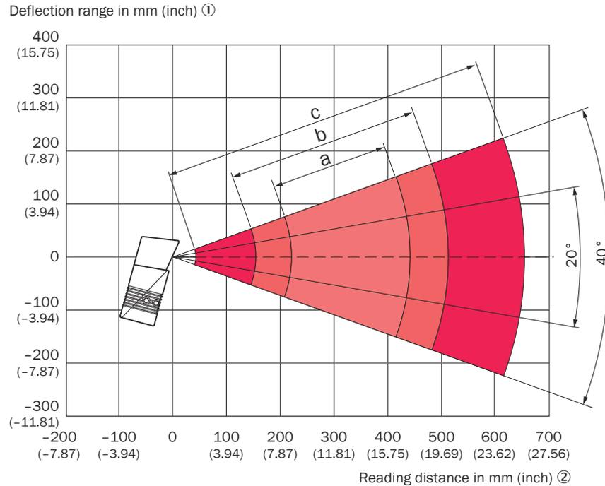
Devices with plastic viewing window: the depth of field is reduced by approx. 10 %. ③
