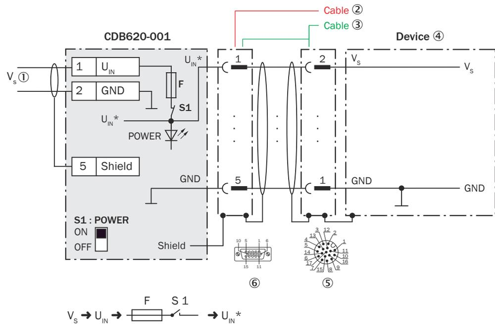
Figure 153: Connecting supply voltage for the device in the CDB620-001 connection module, Ethernet variant with male connector, M12, 17-pin, A-coded
