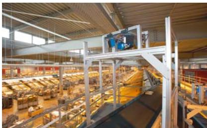
In today's logistics systems, omnidirectional reading tasks are performed using omni port systems (OPS). Powerful and flexible thanks to the use of individual scanners.
