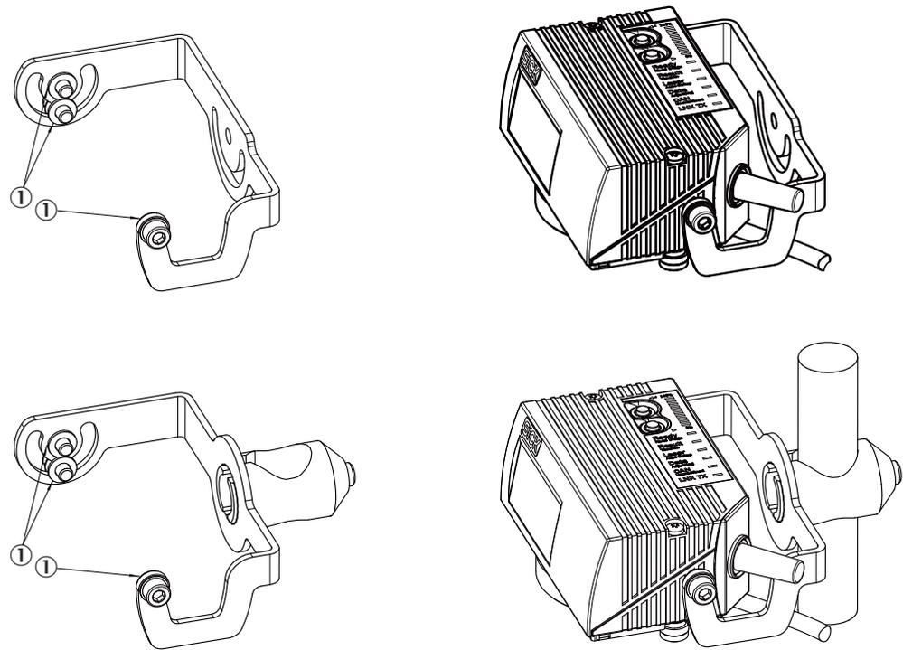
Figure 23: Mounting examples for device with heating: Mounting via bow-shaped mounting bracket (SICK accessories). Illustration of the device may differ.
