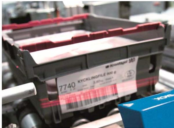
Figure 4: Oscillating mirror scanners read bar codes within a specified range, even in poor lighting conditions.
