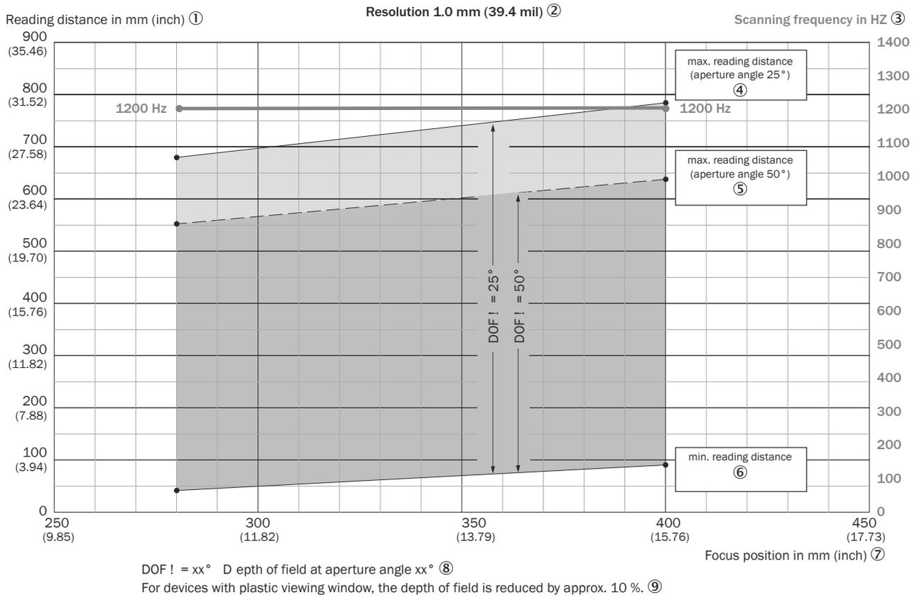
Figure 116: Depth of field ranges for CLV640-Xxx0, line (X = 2) or raster (X = 3), 1.00 mm resolution, glass viewing window, on the side. Minimum and maximum reading distance as a function of focus position and aperture angle
