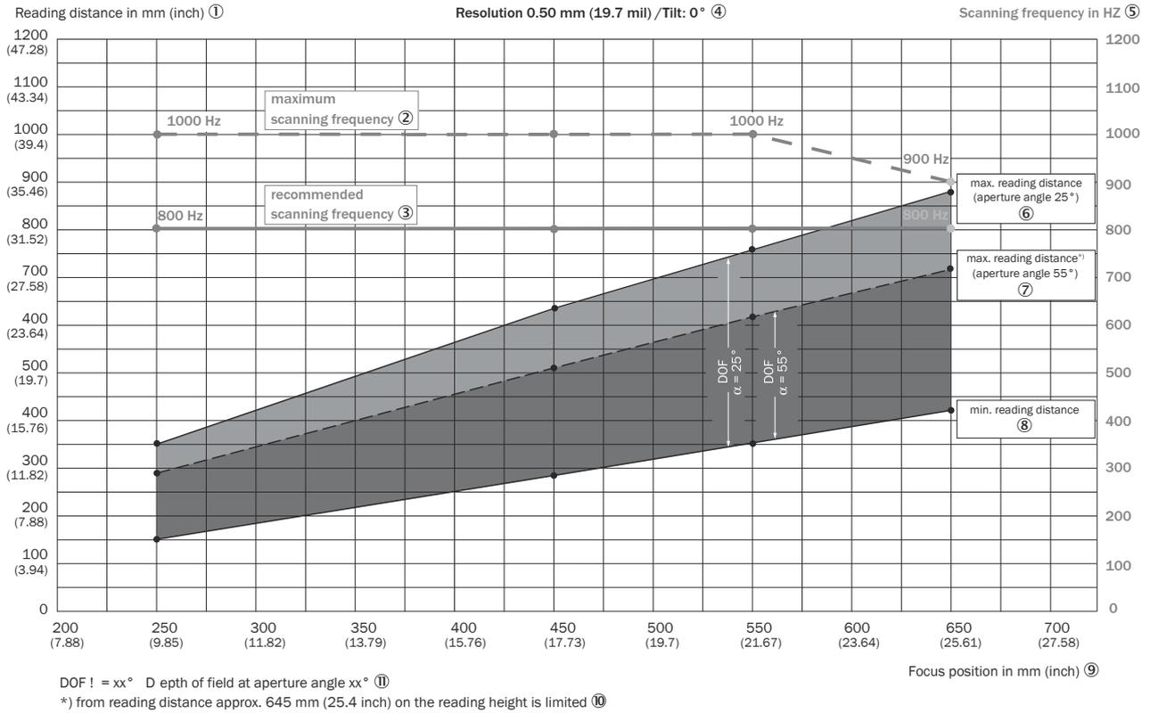
Depth of field ranges of the CLV651 line scanner with oscillating mirror (side reading window: Resolution 0.5 mm (19.7 mil); inclination angle 0°; aperture angle 25°/55°
