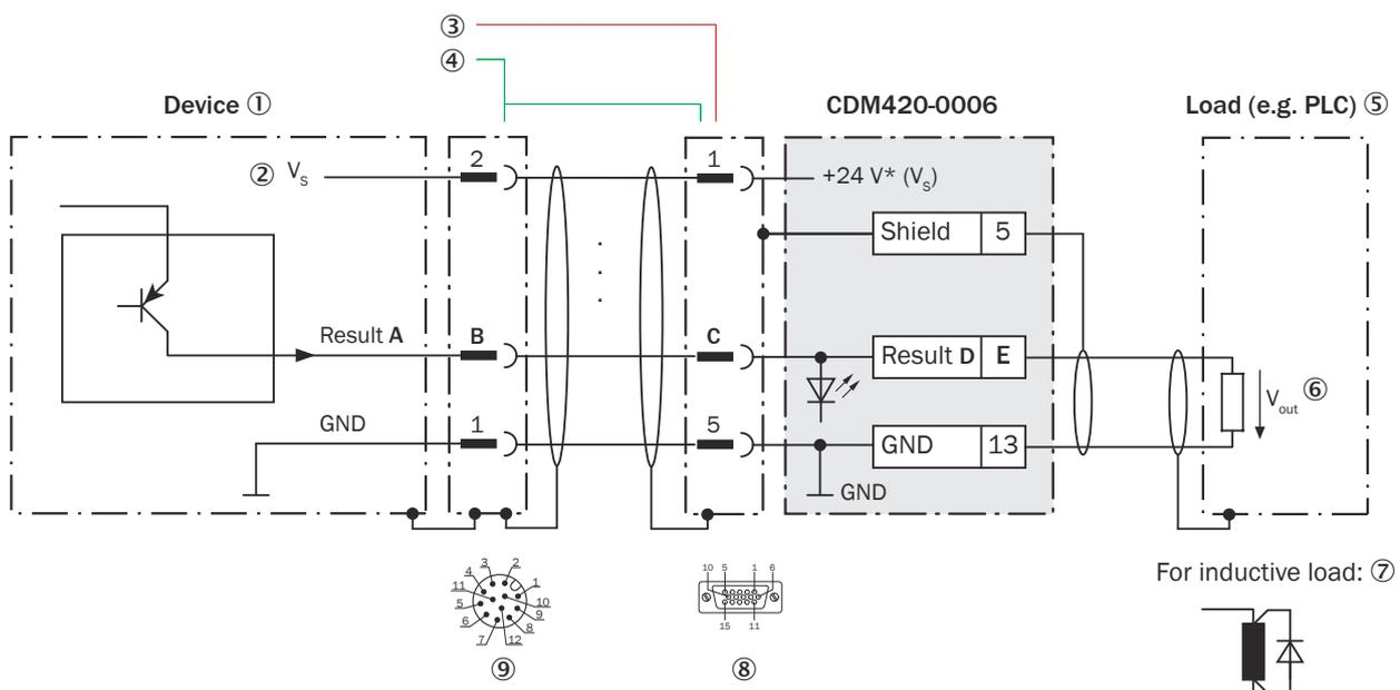
Figure 217: Wiring the “Result 1” and “Result 2” digital outputs of the device in the connection module CDM420-0006, Ethernet variant with male connector, M12, 12-pin, A-coded.
