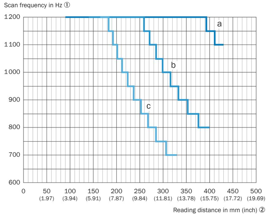
Figure 92: All sensor types: Scanning frequency characteristic curve field for CLV631-xxxx, Mid Range, viewing window at the front
