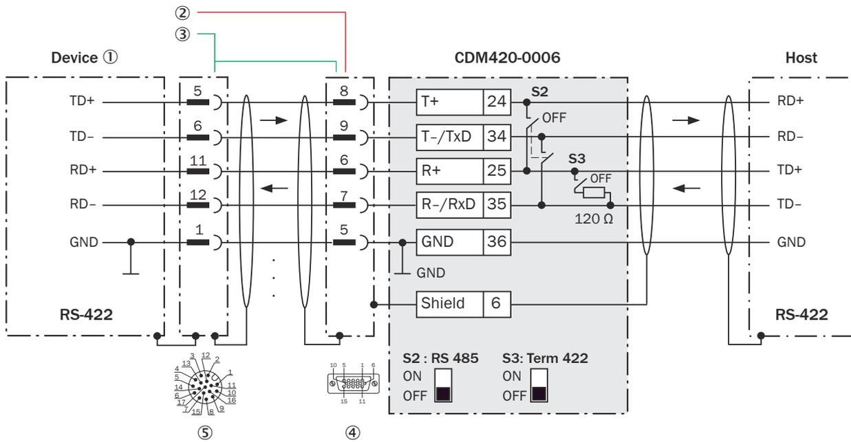
Figure 208: Wiring data interface RS-422 of the device in the CDM420-0006 connection module, Ethernet variant with male connector, M12, 17-pin, A-coded
