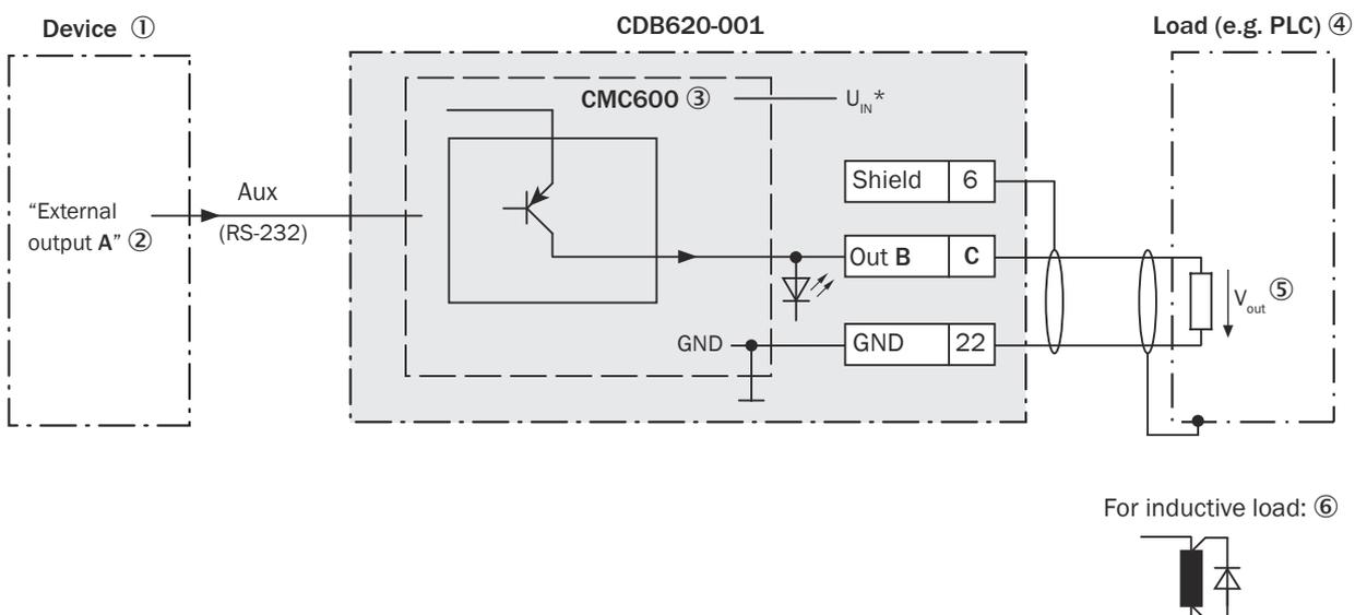
Figure 168: Wiring "Out 1" and "Out 2" external digital outputs of the device in the connection module CDB620-001.
