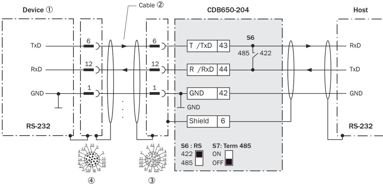
Figure 172: Wiring data interface RS-232 of the device in the connection module CDB650-204
