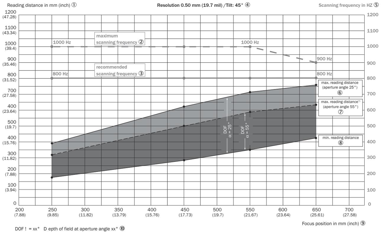
Depth of field ranges of the CLV651 line scanner with front reading window: Resolution 0.5 mm (19.7 mil); inclination angle 45°; aperture angle 25°/55°
