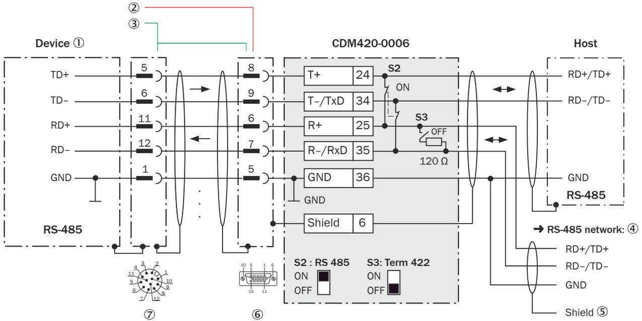
Figure 209: Wiring the RS-485 data interface of the device in the CDM420-0006 connection module, Ethernet variant with male connector, M12, 12-pin, A-coded.
