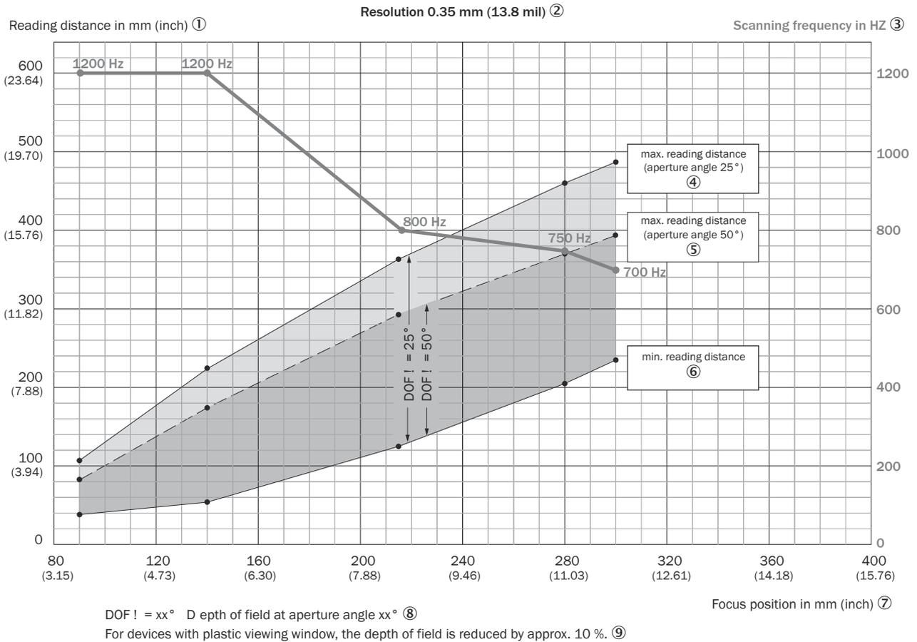
Figure 114: Depth of field ranges for CLV640-Xxx0, line (X = 2) or raster (X = 3), 0.35 mm resolution, glass viewing window, on the side. Minimum and maximum reading distance as a function of focus position and aperture angle
