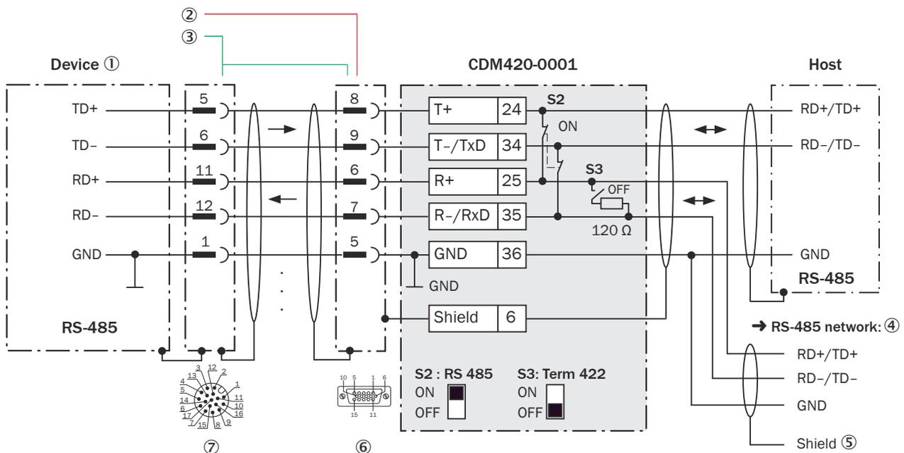
Figure 191: Wiring the RS-485 data interface of the device in the CDM420-0001 connection module, Ethernet variant with male connector, M12, 17-pin, A-coded
