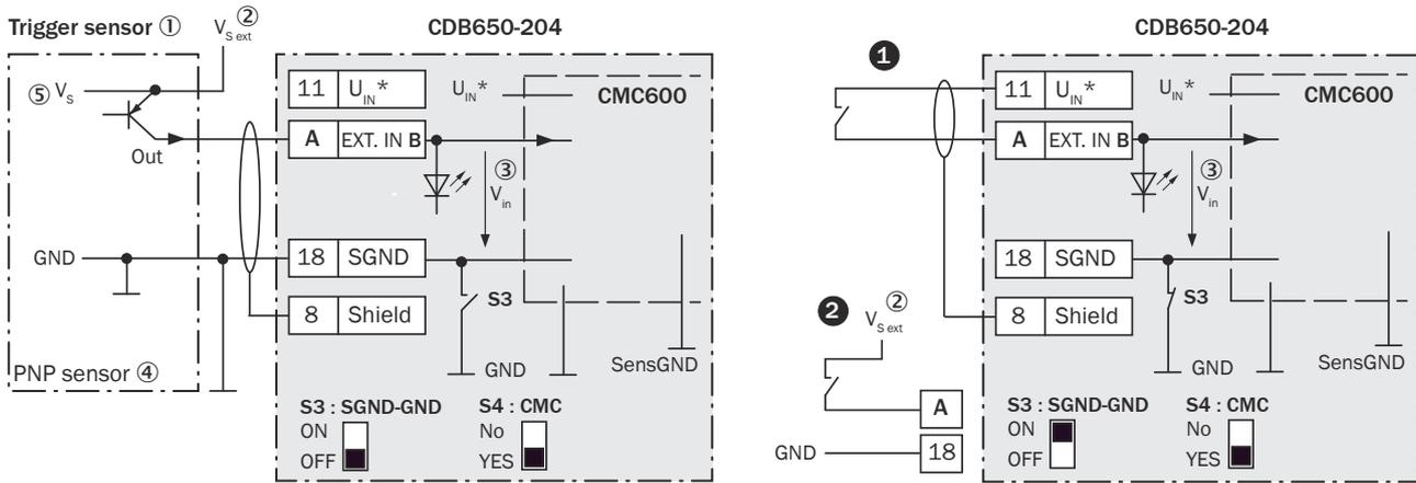
Figure 179: Left: Trigger sensor connected potential-free and supplied with power externally. Right: Alternatively switch, ❶ supplied with power by connection module CDB650-204 or ❷ connected potential-free and supplied with power externally. Switch setting S3 then as in left figure.
