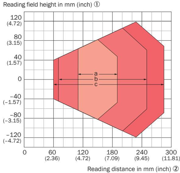
Figure 93: Reading field diagram for CLV632-Xxx0, short range, line scanner (X = 0) or raster scanner (X = 1), glass viewing window, at the front
