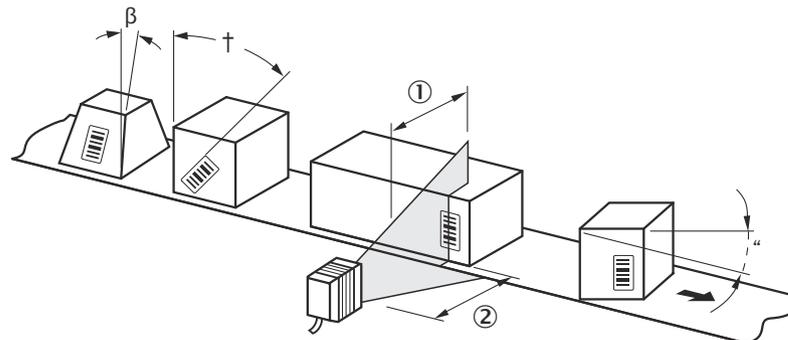
Figure 25: Line scanner: Occurring reading angle between scan line and bar code
