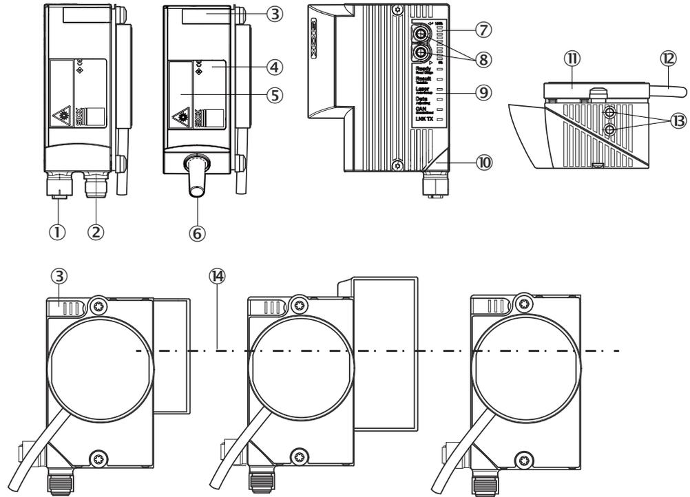
Figure 11: Device variants CLV63x to CLV65x with heating: Overview of components
