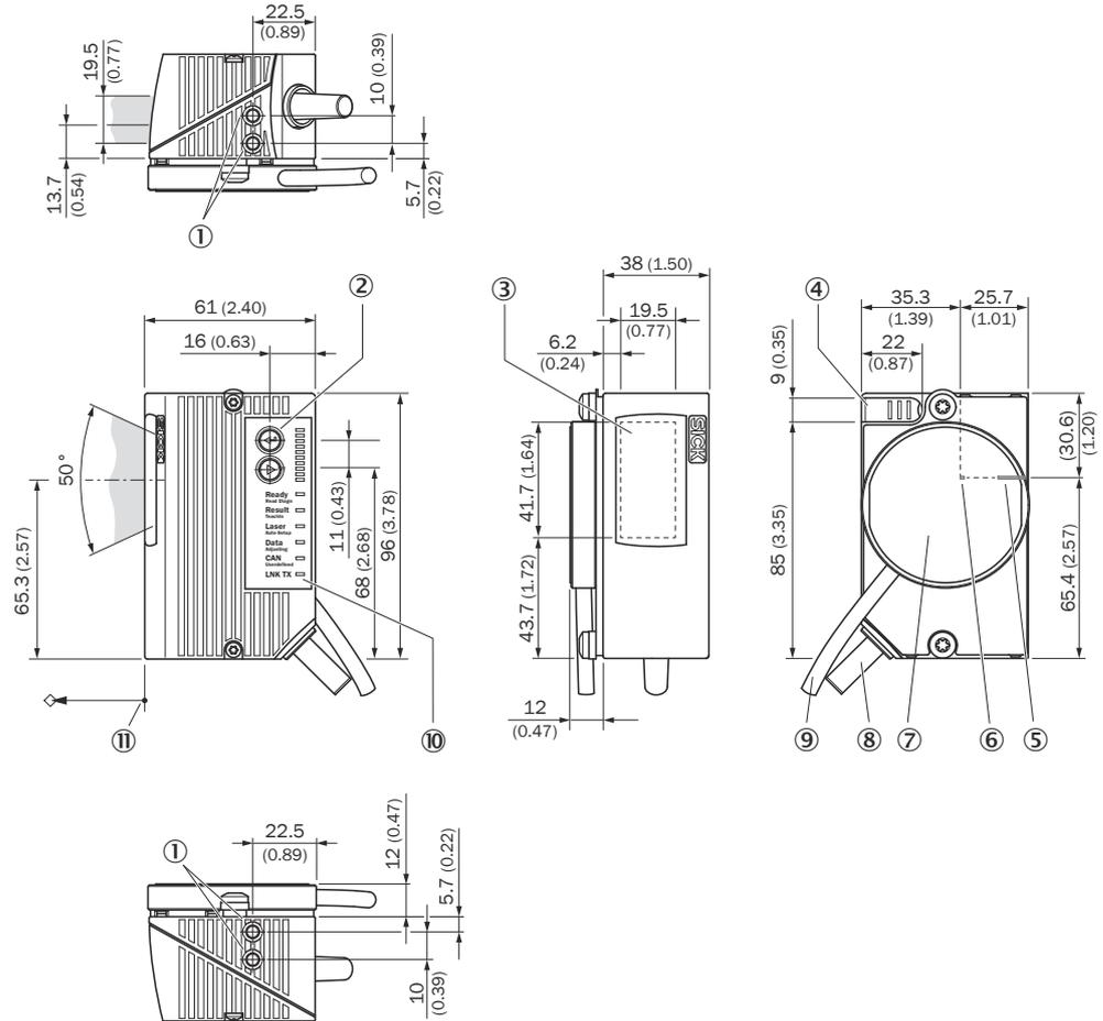
Figure 76: CLV63x to CLV65x: Serial variant in standard housing with external heating, front viewing window and connecting cable. structure and device dimensions, unit: mm (inch), decimal separator: period
