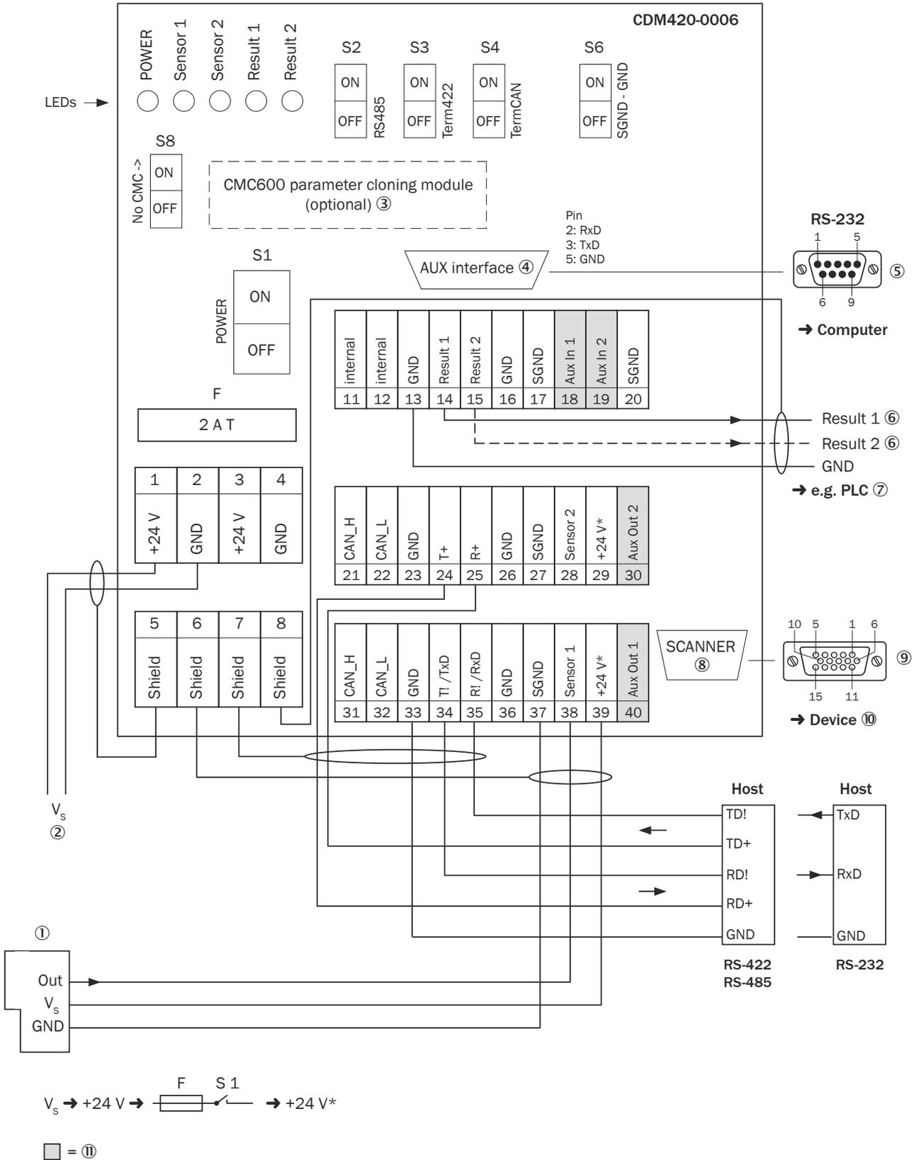
Figure 202: Overview: connection of device (without heating) and peripherals to the CDM420-0006 connection module
