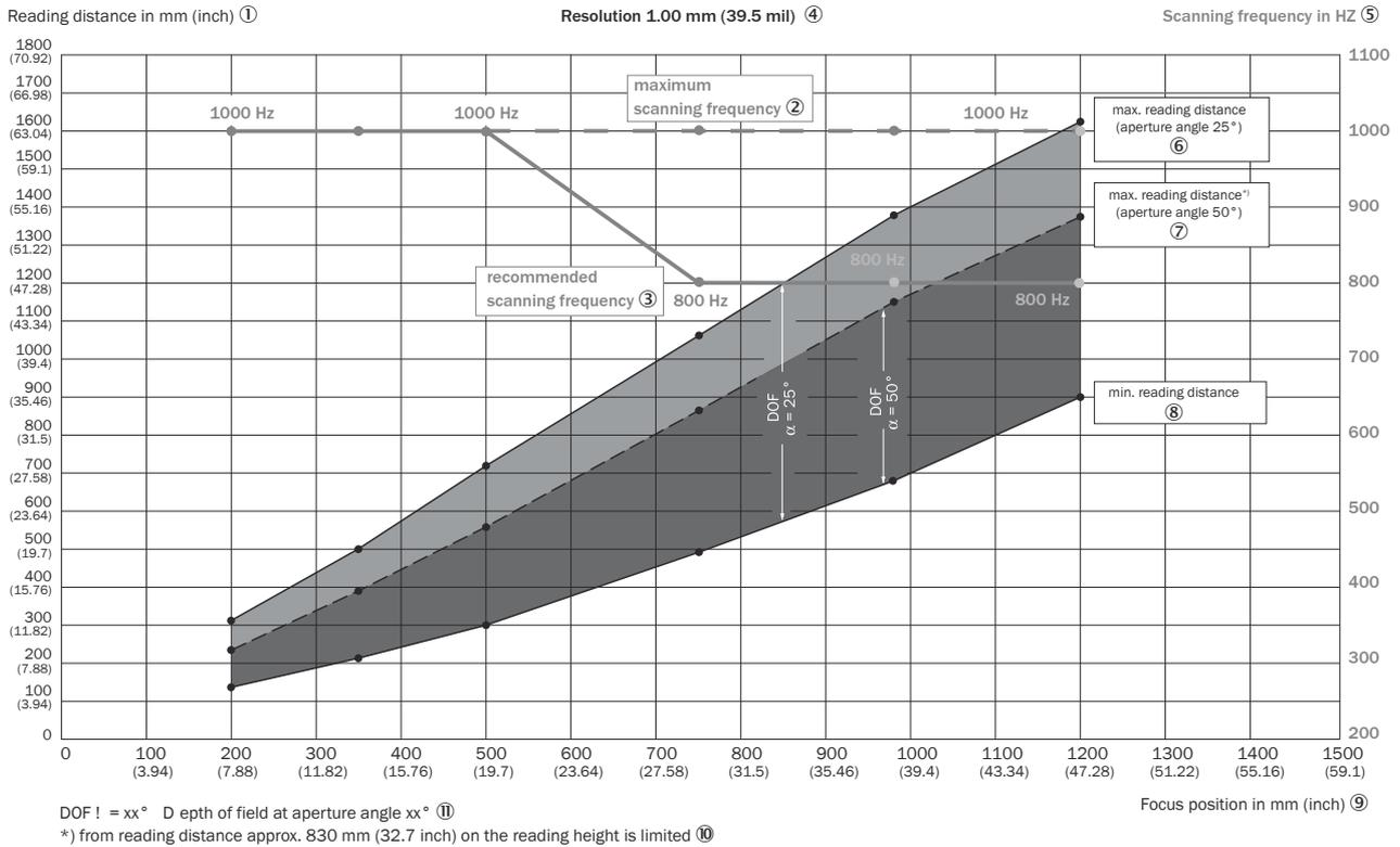
Depth of field ranges of the CLV650 line scanner with front reading window: Resolution 1.00 mm (39.5 mil)
