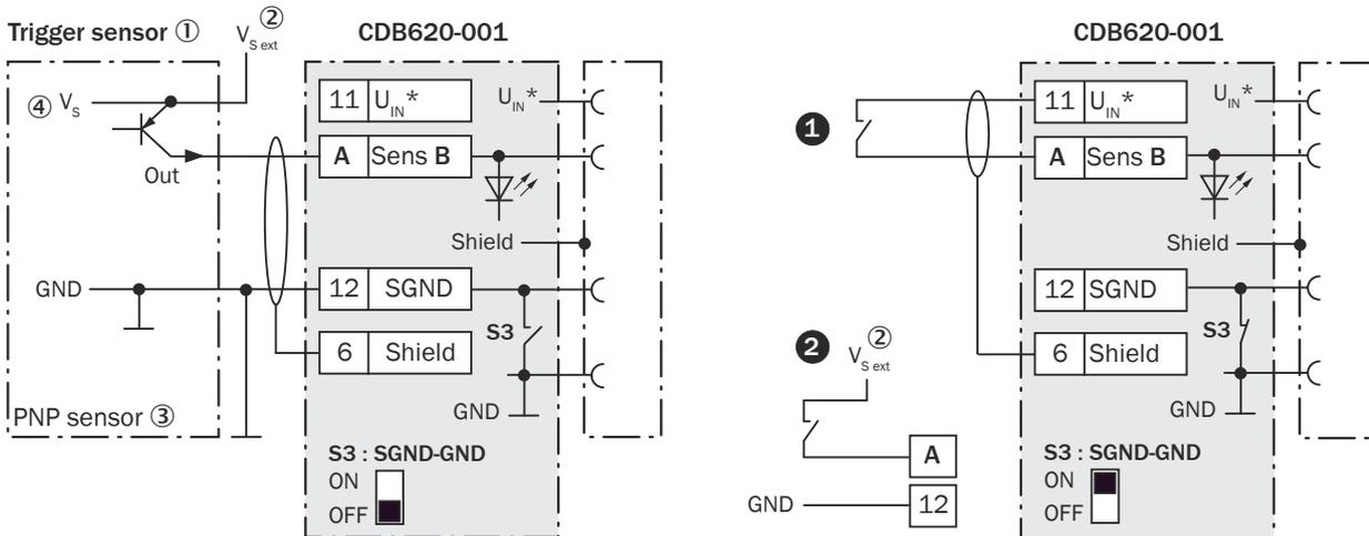
Figure 163: Left: Trigger sensor connected potential-free and supplied with power externally. Right: alternative switch, ① supplied with power by connection module CDB620-001 or ② connected volt-free and supplied with power externally. Now select switch setting S3 as shown in the left figure.
