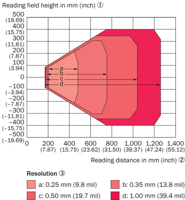
Figure 126: Reading field diagram for CLV650-0120S01, standard density, line, glass viewing window, at the front, with polarizing filter
