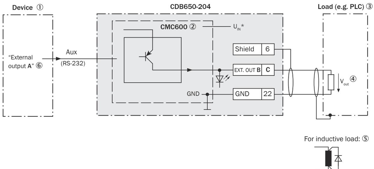
Figure 181: Wiring external "External output 1" and "External output 2" digital outputs of the device in the CDB650-204 connection module.
