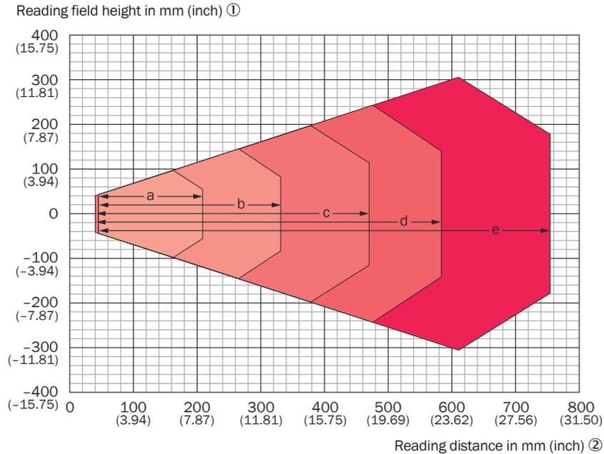
For devices with plastic reading window (CLV640-6120S01, CLV640-6831S01 and CLV640-6121S01): the depth of field is reduced by approx. 10%. ③
