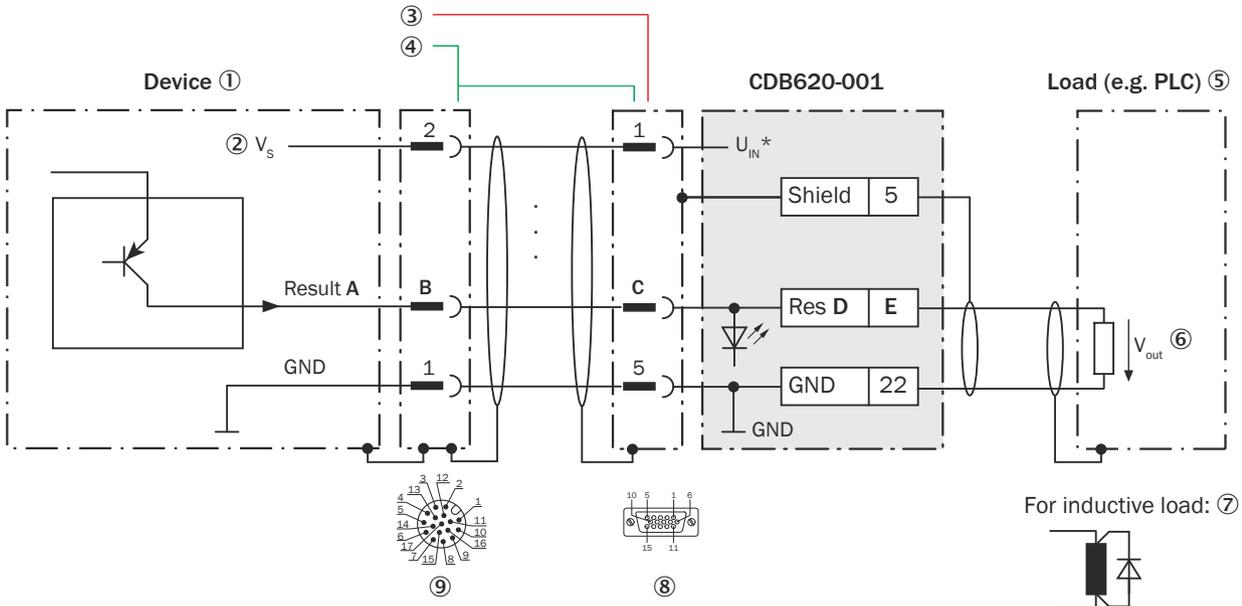
Figure 167: Wiring the “Result 1” and “Result 2” digital outputs of the device in the connection module CDB620-001, Ethernet variant with male connector, M12, 17-pin, A-coded.
