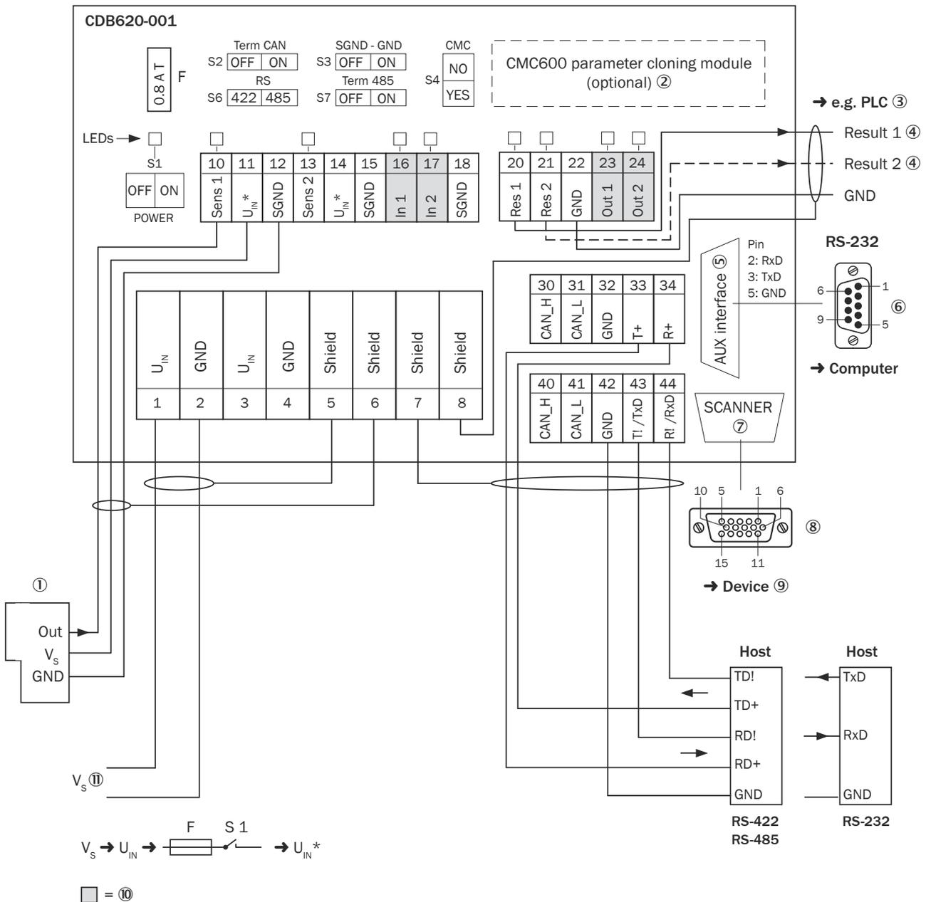
Figure 151: Overview: connection of device (without heating) and peripherals to the CDB620-001 connection module.
