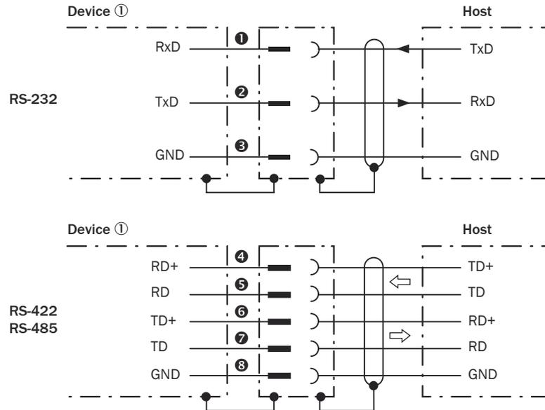
Figure 51: Internal circuitry for data interfaces: RS-232 and RS-422/485
