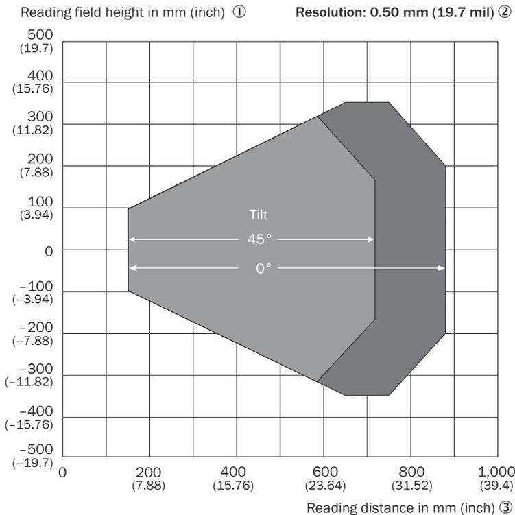
Figure 132: Reading field diagram for CLV651-6xx0, low density, line with oscillating mirror, glass viewing window, on the side, tilt angle 45° and 0°
