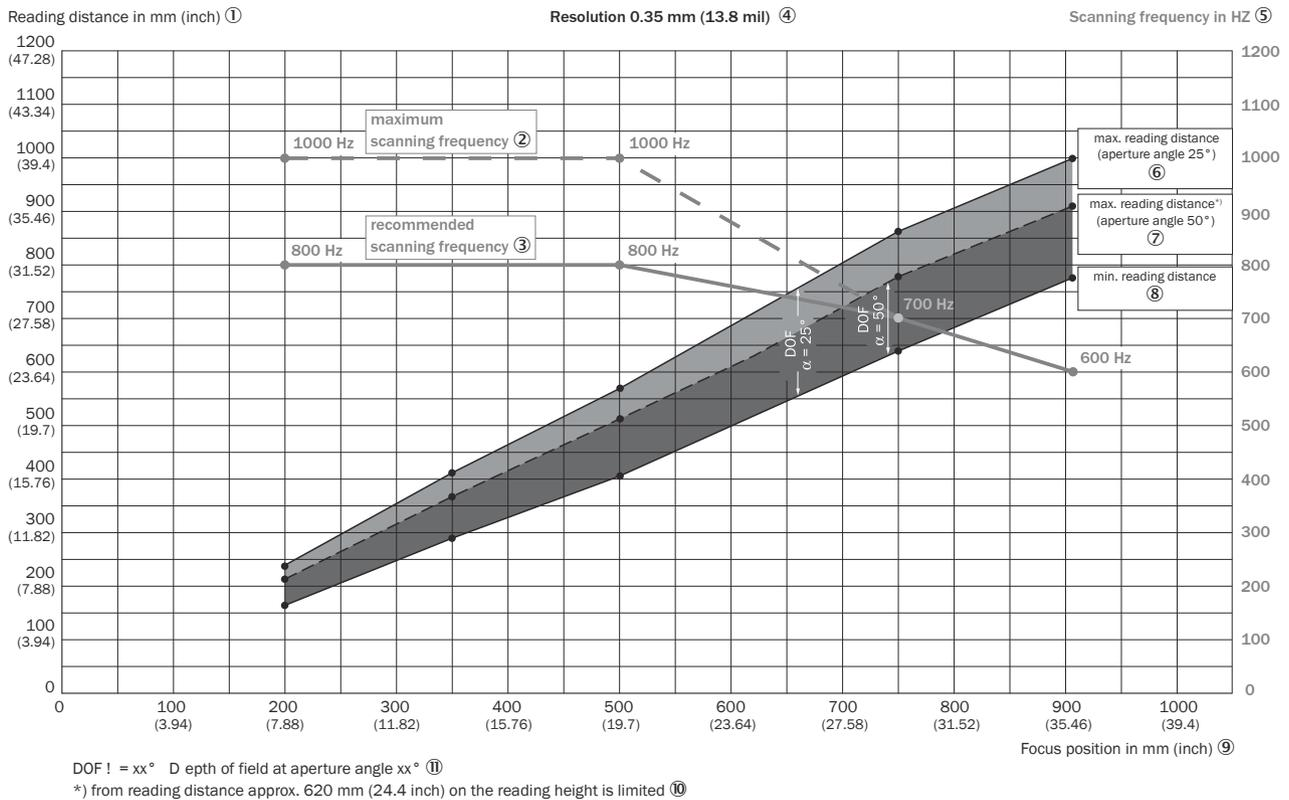
Depth of field ranges of the CLV650 line scanner with front reading window: Resolution 0.35 mm (13.8 mil)
