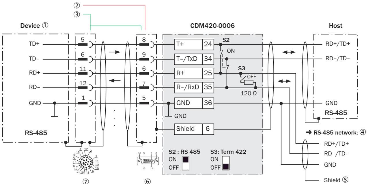
Figure 210: Wiring the RS-485 data interface of the device in the CDM420-0006 connection module, Ethernet variant with male connector, M12, 17-pin, A-coded.
