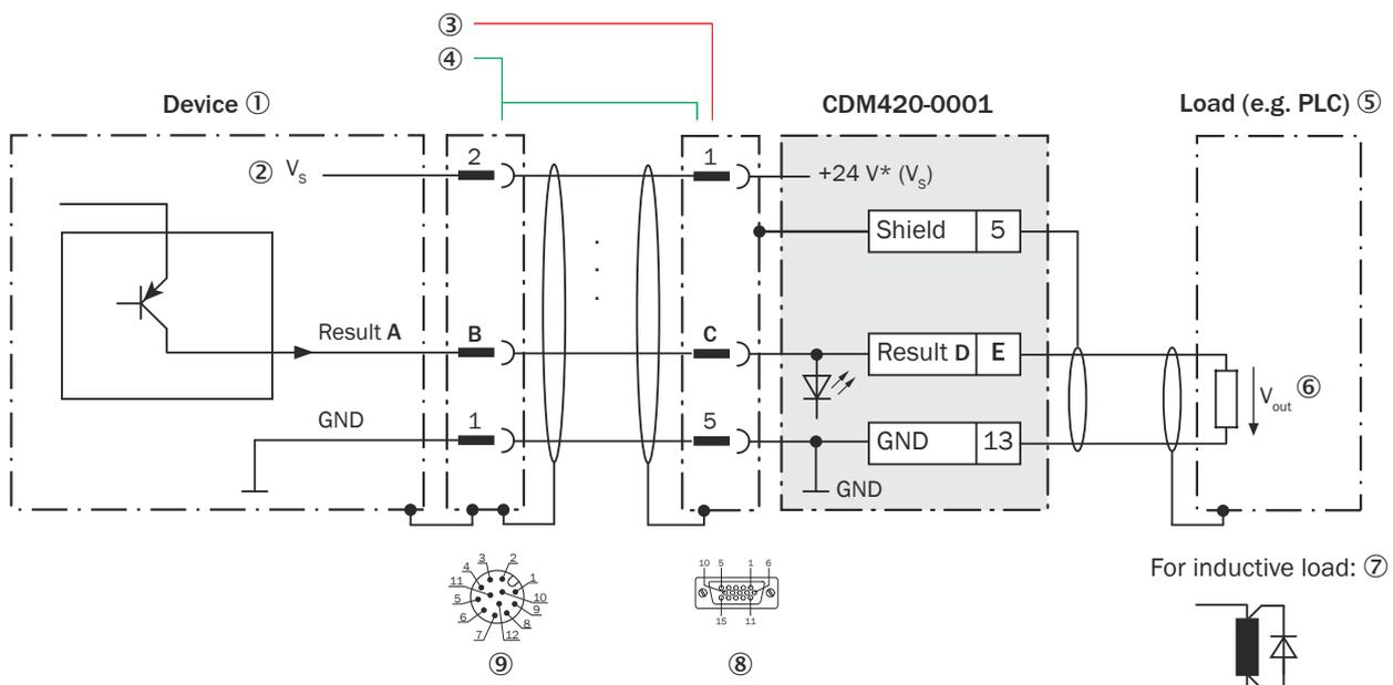
Figure 198: Wiring the digital outputs “Result 1” and “Result 2” of the device in the connection module CDM420-0001, Ethernet variant with male connector, M12, 12-pin, A-coded
