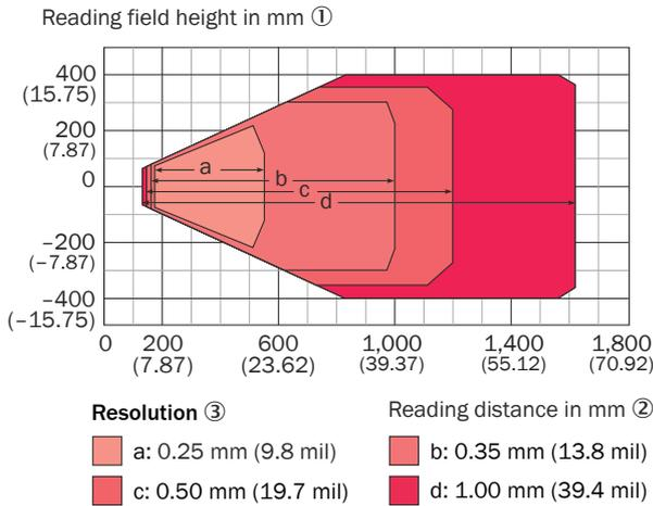
Figure 125: Reading field diagram for CLV650-Xxx0, standard density, line (X = 0), glass viewing window, at the front
