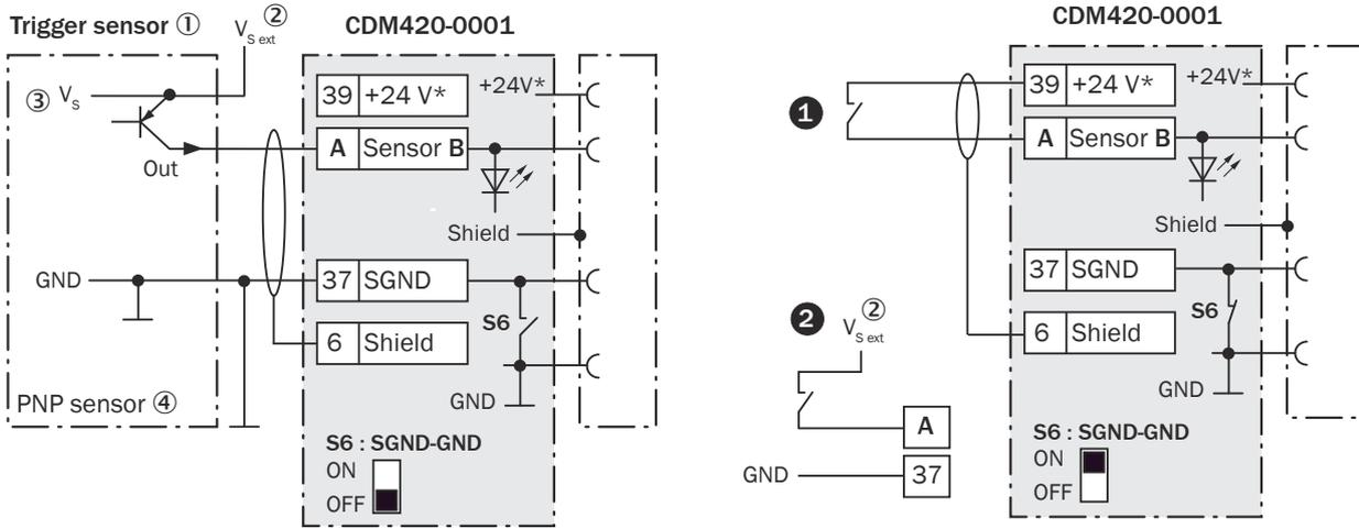
Figure 195: Left: Trigger sensor connected potential-free and supplied with power externally. Right: alternative switch, ❶ supplied with power by connection module CDM420-0001 or ❷ connected volt-free and supplied with power externally. Now select switch setting S6 as shown in the left figure.
