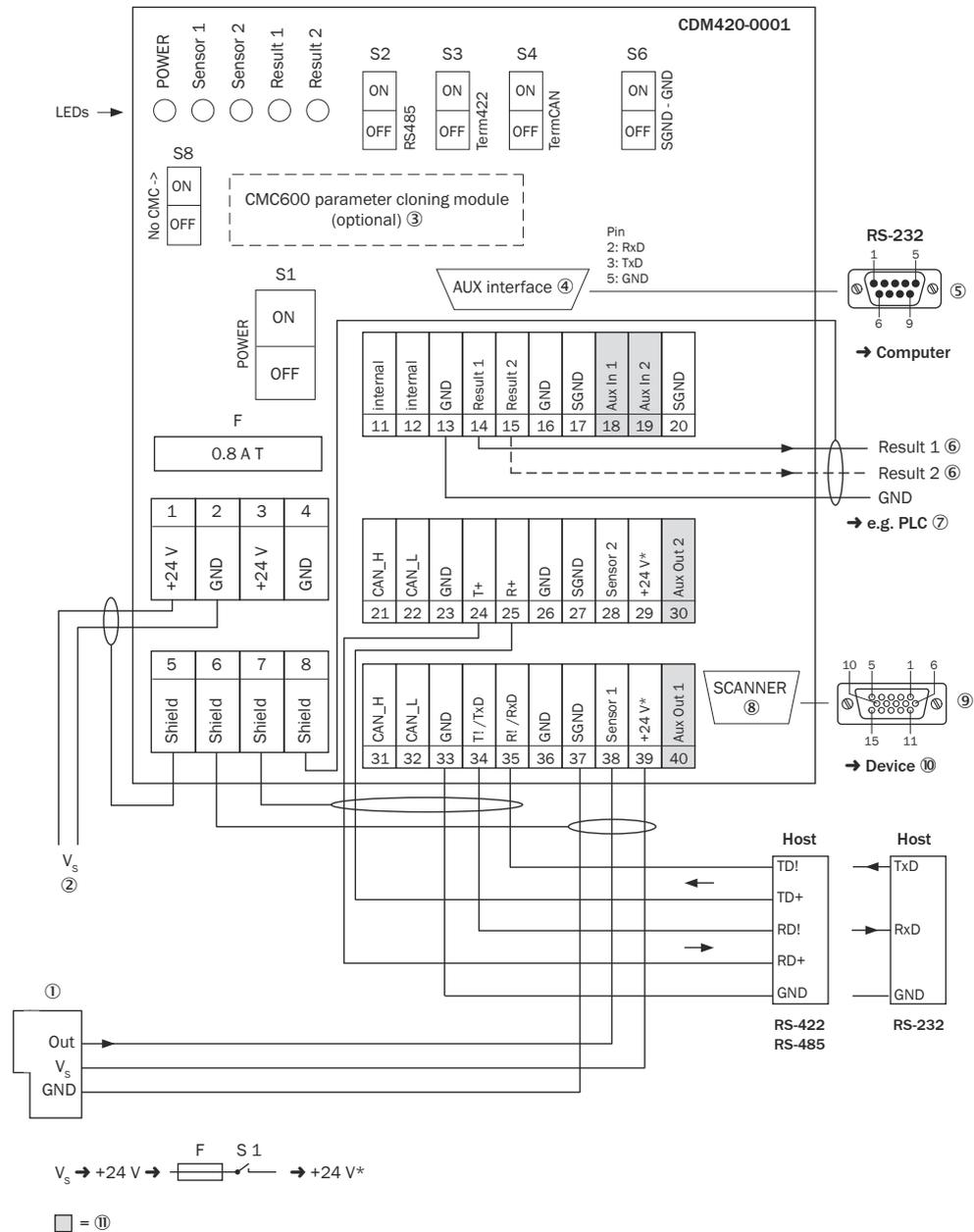
Figure 183: Overview: connection of device (without heating) and peripherals to the CDM420-0001 connection module
