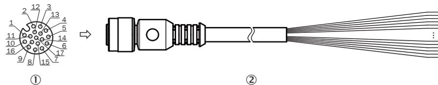
Figure 62: Adapter cable, e.g., part no. 2070425 (3 m)
