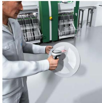
Mobile identification at pick-and-place setup stations
