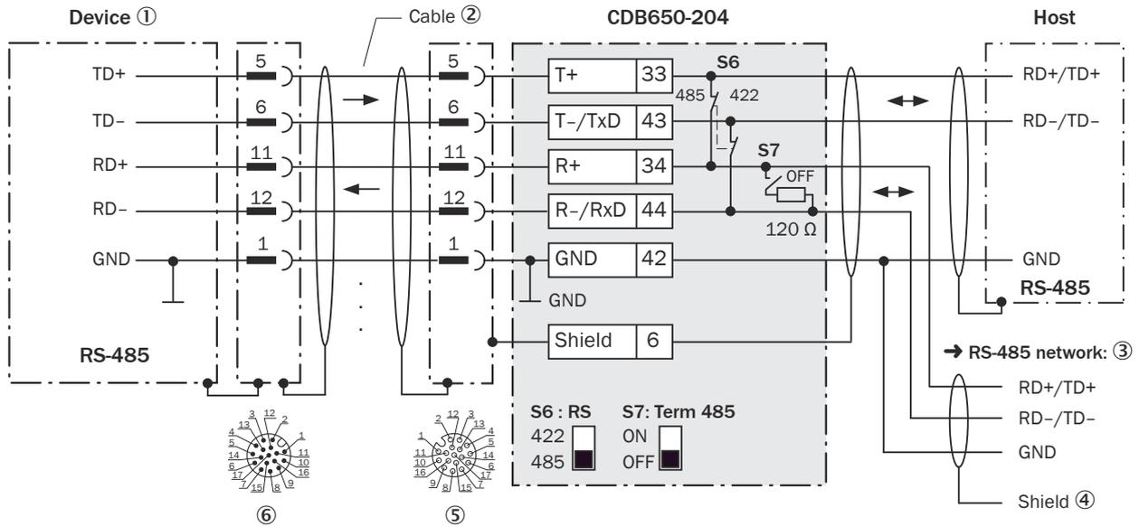
Figure 174: Wiring data interface RS-485 of the device in connection module CDB650-204.
