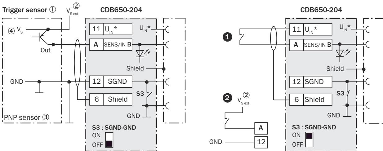
Figure 177: Left: Trigger sensor connected potential-free and supplied with power externally. Right: Alternatively switch, ① supplied with power by connection module CDB650-204 or ② connected potential-free and supplied with power externally. Now select switch setting S3 as shown in the left figure.
