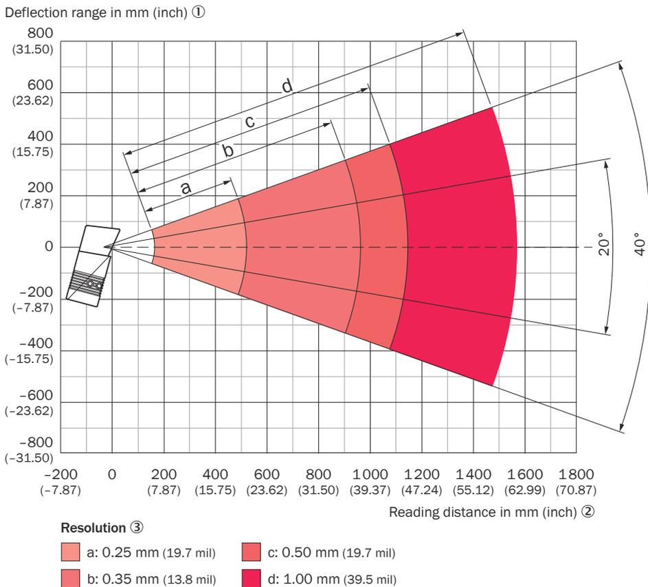
Figure 128: Oscillating mirror deflection width diagram for CLV650-6xx0, standard density, line with oscillating mirror, glass viewing window, on the side
