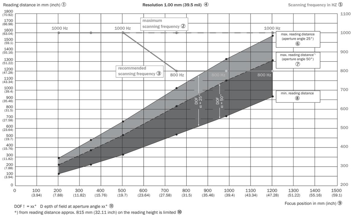
Depth of field ranges of the CLV650 line scanner with oscillating mirror: Resolution 1.00 mm (39.5 mil)
