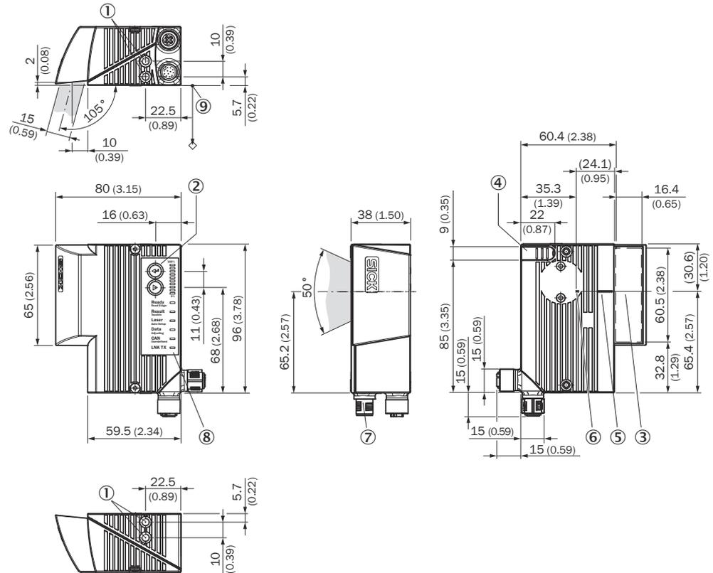
Figure 68: CLV63x to CLV65x: Ethernet variant in standard housing, with side viewing window and swivel connector. structure and device dimensions, unit: mm (inch), decimal separator: period
