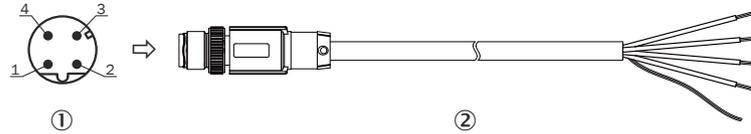
Figure 65: Adapter cable, e.g. part no. 2106171 (2 m)
