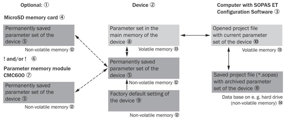
Figure 54: Configuration with SOPAS ET and saving the parameter set
