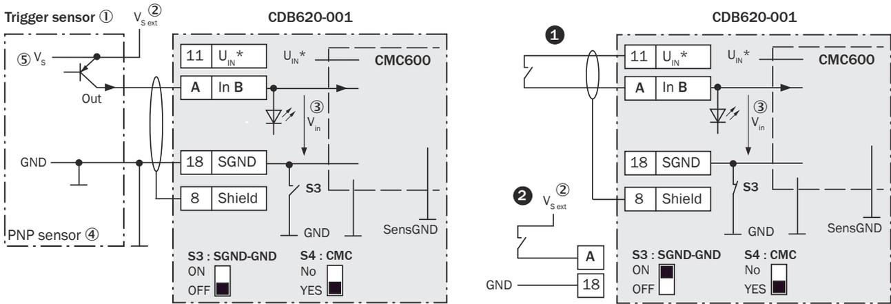
Figure 165: Left: Trigger sensor connected potential-free and supplied with power externally. Right: alternative switch, ❶ supplied with power by connection module CDB620-001 or ❷ connected volt-free and supplied with power externally. Now select switch setting S3 as shown in the left figure.
