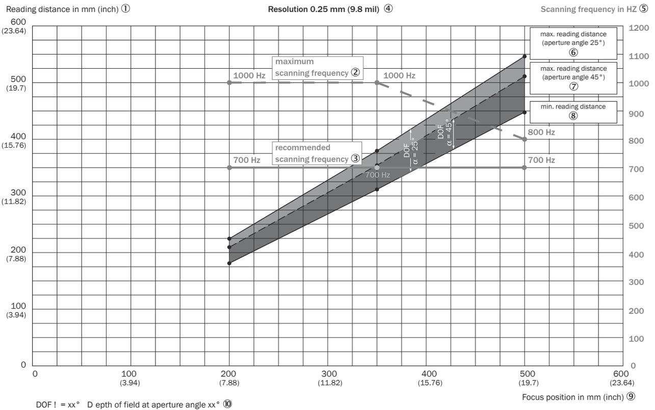
Figure 134: Depth of field ranges of the CLV650-1xx0, line scanner (line), 0.25 mm resolution, glass viewing window, at the front. Minimum and maximum reading distance as a function of focus position and aperture angle
