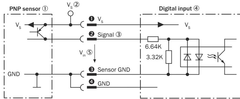
Figure 52: Wiring of a digital input on the device with external PNP sensor
