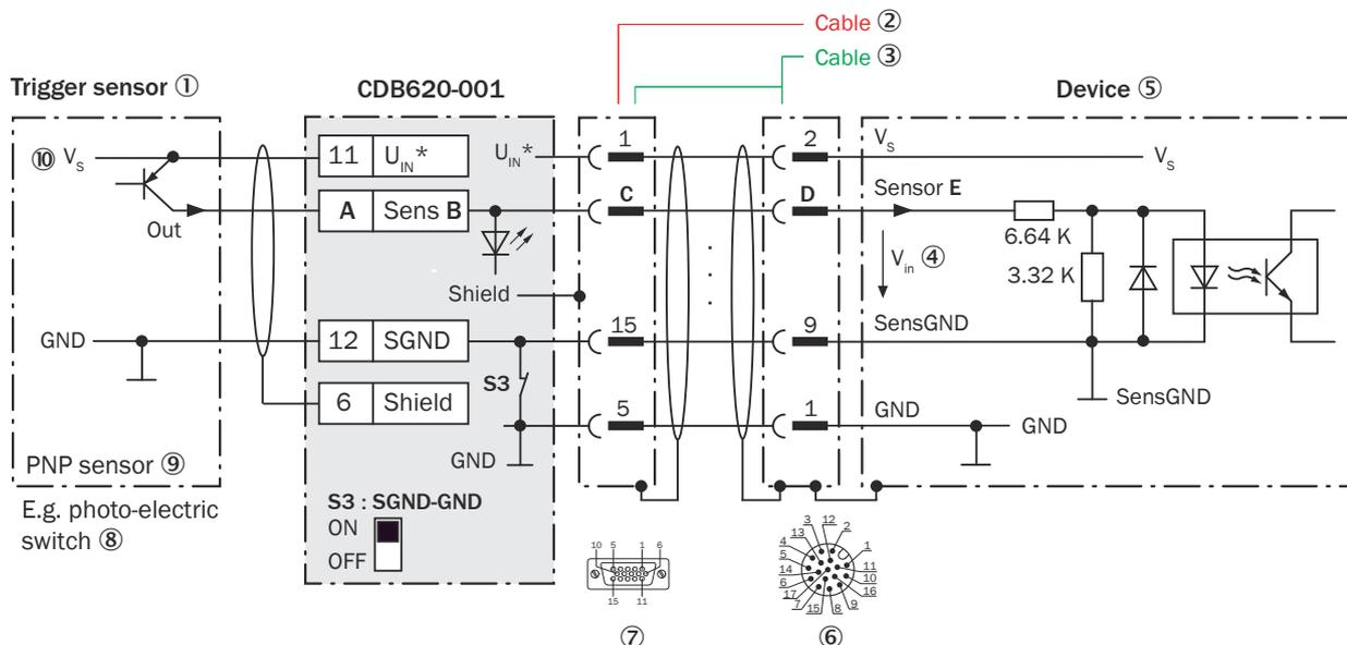
Figure 162: Trigger sensor supplied with power by connection module CDB620-001, Ethernet variant with male connector, M12, 17-pin, A-coded
