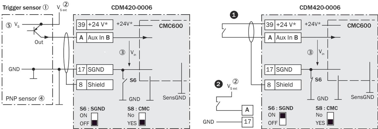
Figure 216: Left: Trigger sensor connected potential-free and supplied with power externally. Right: Alternatively switch, ❶ supplied with power by connection module CDM420-0006 or ❷ connected potential-free and supplied with power externally. Switch setting S3 then as in left figure.
