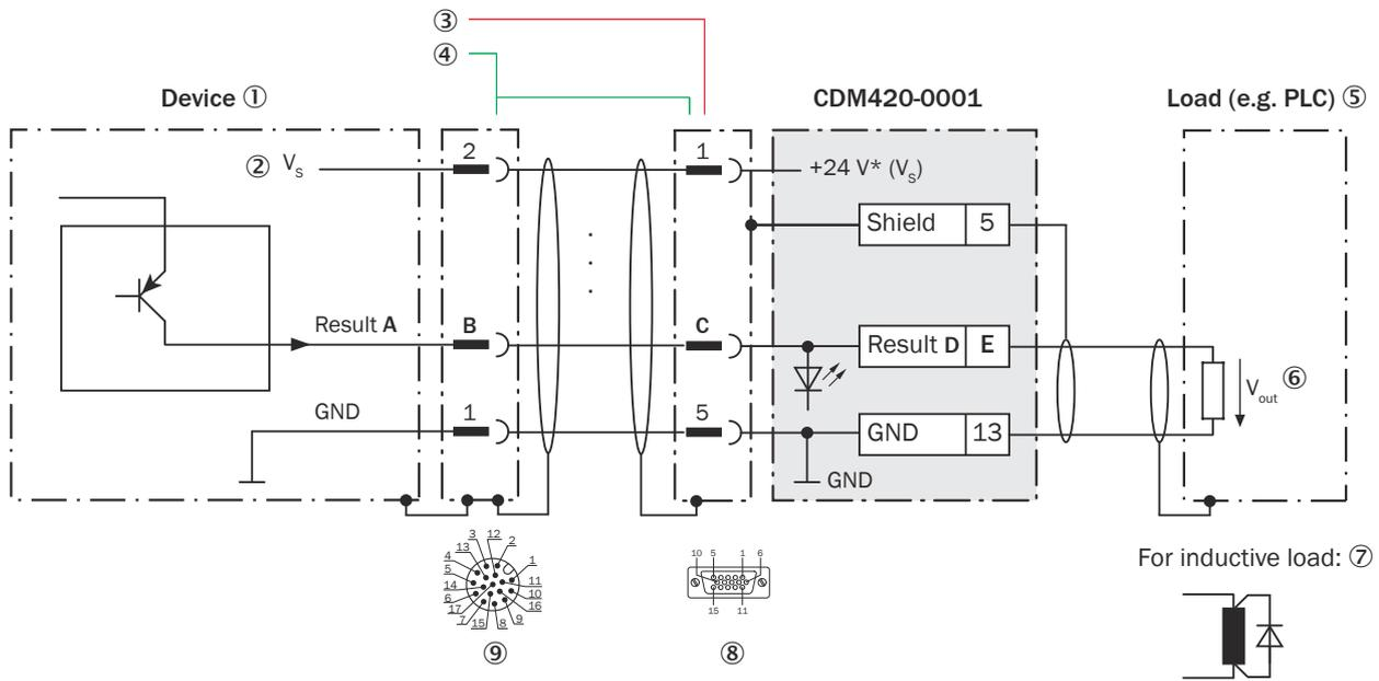
Figure 199: Wiring the “Result 1” and “Result 2” digital outputs of the device in the connection module CDM420-0001, Ethernet variant with male connector, M12, 17-pin, A-coded.
