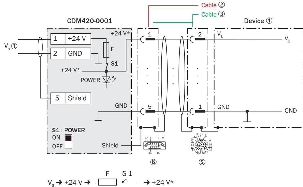
Figure 185: Connecting supply voltage for the device in the CDM420-0001 connection module, Ethernet variant with male connector, M12, 17-pin, A-coded
