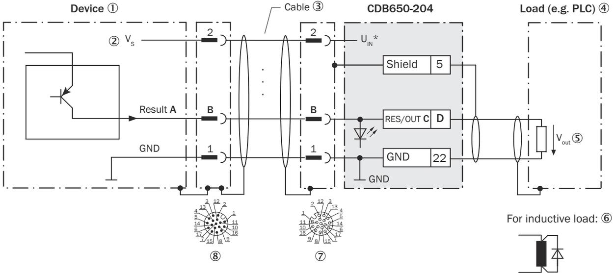
Figure 180: Wiring the digital outputs “Result 1” and “Result 2” of the device in the connection module CDB650-204
