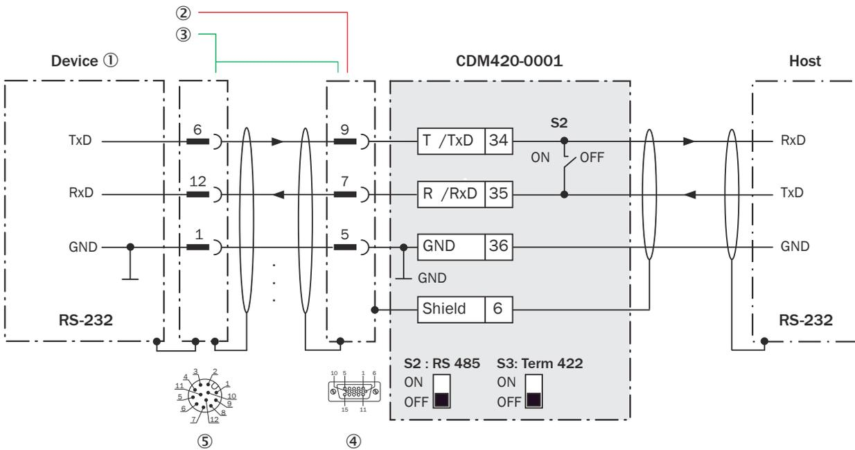
Figure 186: Wiring data interface RS-232 of the device in the CDM420-0001 connection module, Ethernet variant with male connector, M12, 12-pin, A-coded
