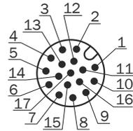
Figure 44: Male connector, M12, 17-pin, A-coded
