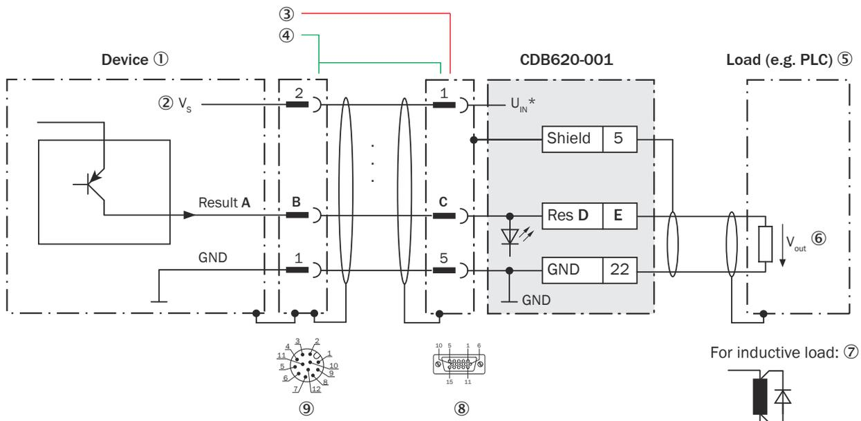
Figure 166: Wiring the digital outputs "Result 1" and "Result 2" of the device in the connection module CDB620-001, Ethernet variant with male connector, M12, 12-pin, A-coded
