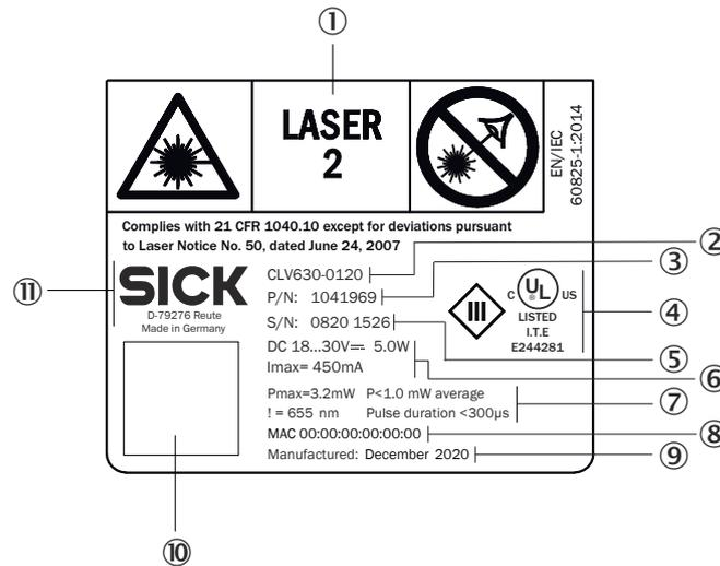
Figure 5: CLV63x, CLV64x and CLV65x: Example of type label for CLV630-0120 (serial variant). For devices in IP65 standard housing. Electrical values shown here for devices without heating. Figure may differ.
