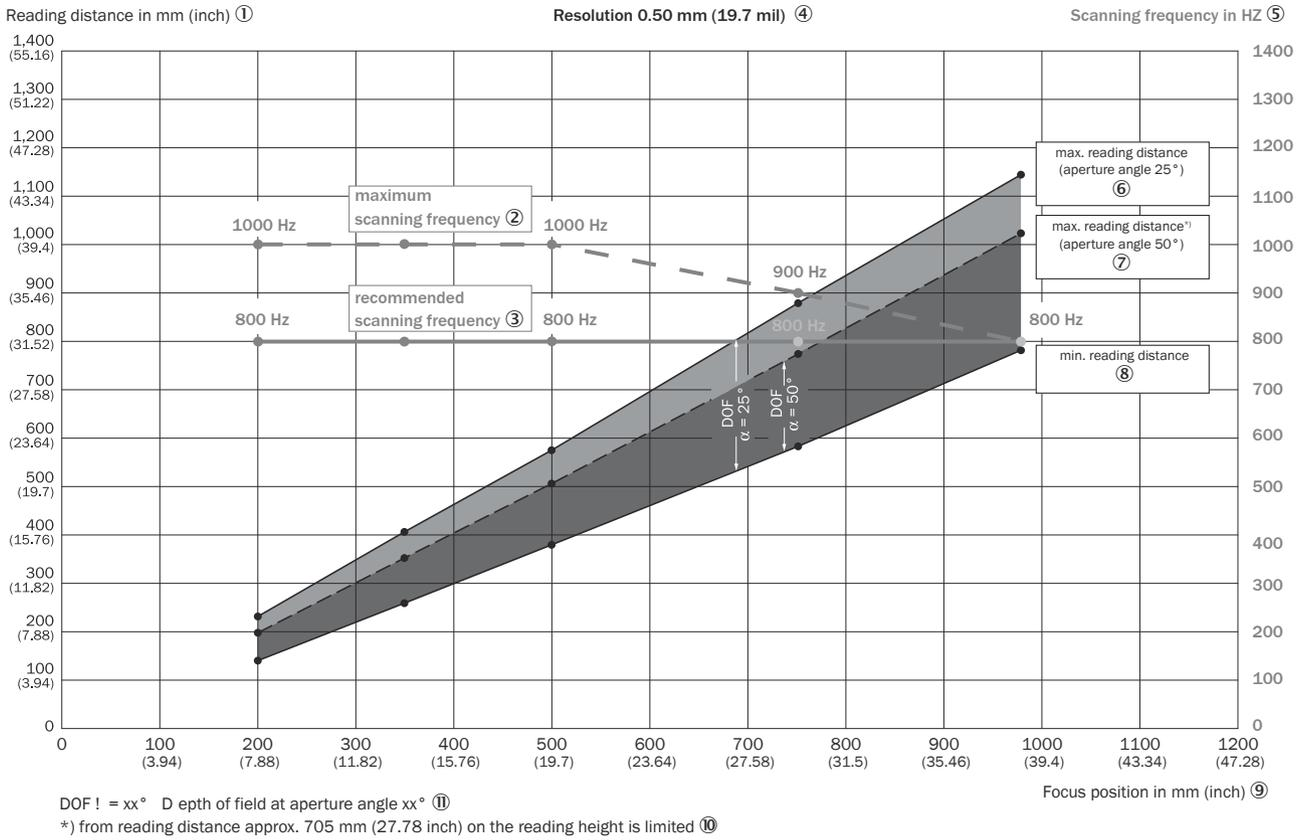
Depth of field ranges of the CLV650 line scanner with oscillating mirror: Resolution 0.50 mm (19.7 mil)
