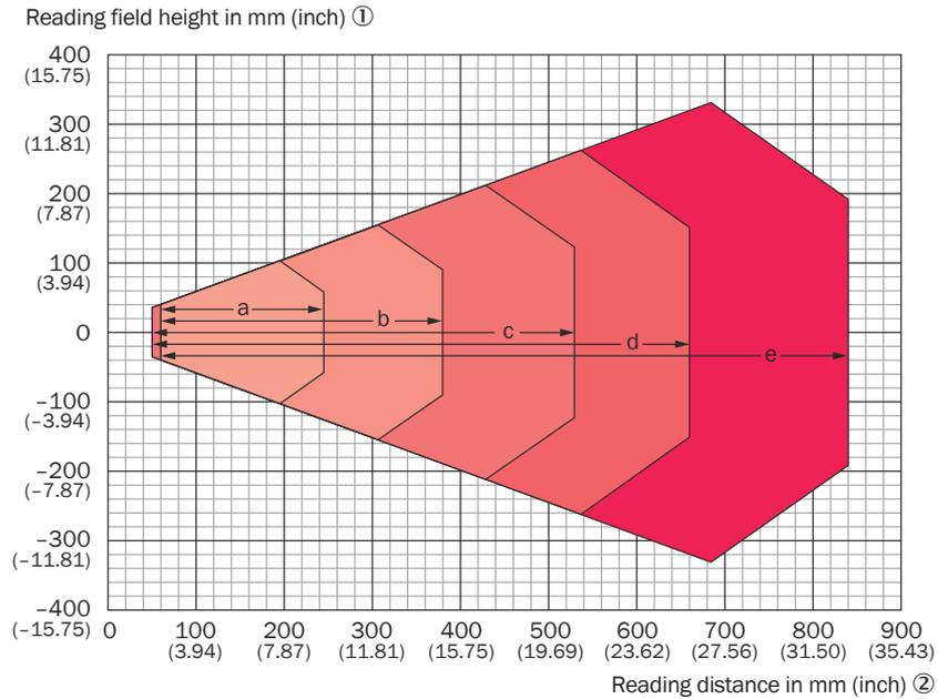
For devices with plastic reading window (CLV640-0831S01):
