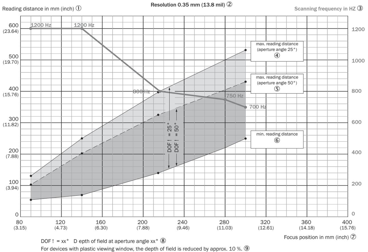
Figure 109: Depth of field ranges for CLV640-Xxx0, line (X = 0) or raster (X = 1), 0.35 mm resolution, glass viewing window, at the front. Minimum and maximum reading distance as a function of focus position and aperture angle
