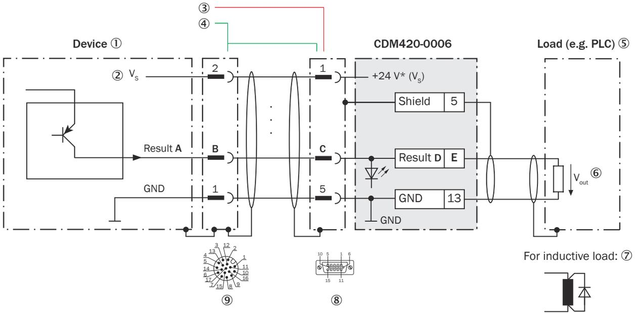
Figure 218: Wiring the digital outputs “Result 1” and “Result 2” of the device in the connection module CDM420-0006, Ethernet variant with male connector, M12, 17-pin, A-coded
