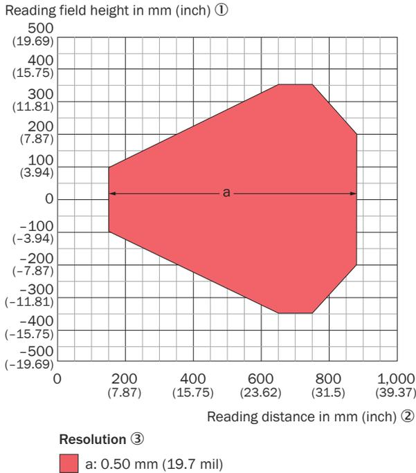
Figure 131: Reading field diagram for CLV651-6xx0, low density, line with oscillating mirror, glass viewing window, on the side
