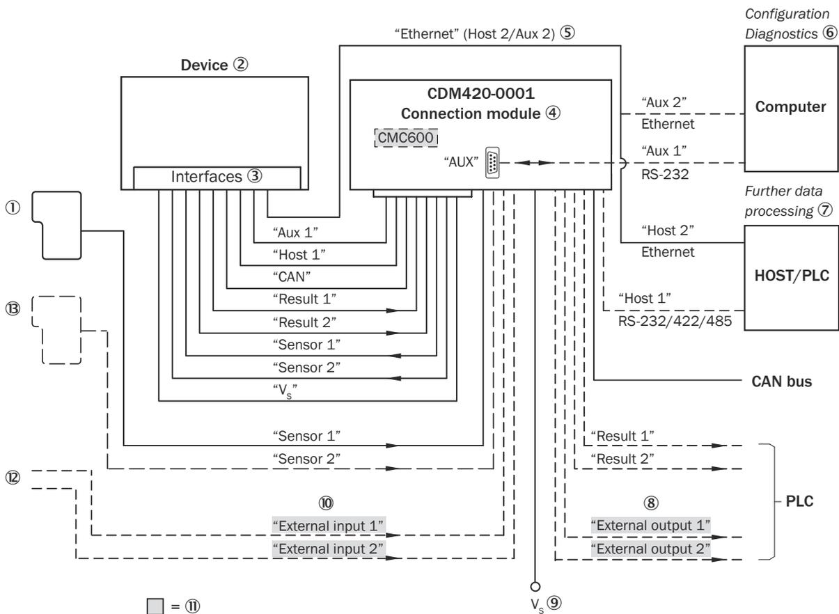
Figure 182: Connection of the device to peripherals via CDM420-0001 (overview)
