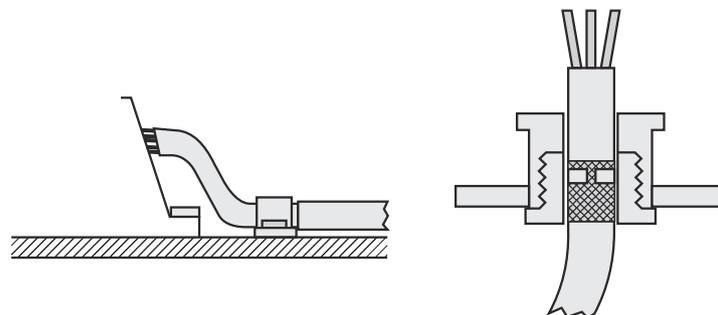
Figure 41: Shield connection in plastic housings
