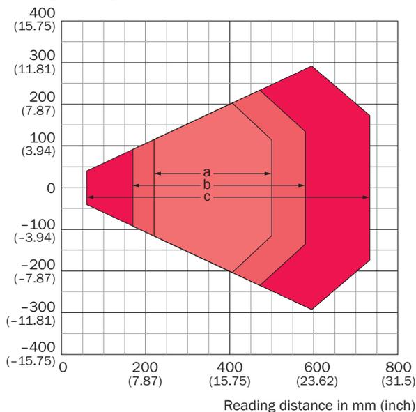
For devices with plastic reading window, the depth of field is reduced by approx. 10 %.
