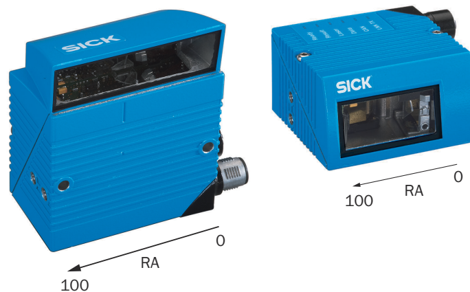
Figure 22: Counting direction of the reading angle RA in the scan plane: For devices in the IP65 standard housing with side viewing window (left) and front viewing window (right)
