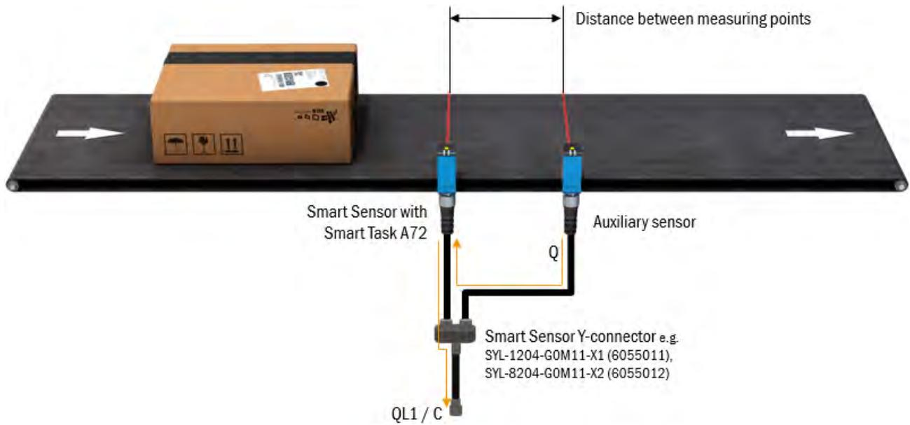
Figure 8: Wiring example for “Length” and “Speed” measurement modes
