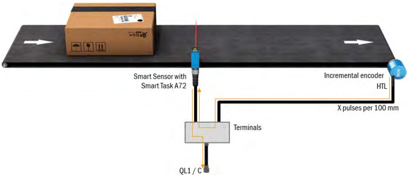
Figure 9: Wiring example for “Length incremental” measurement mode
