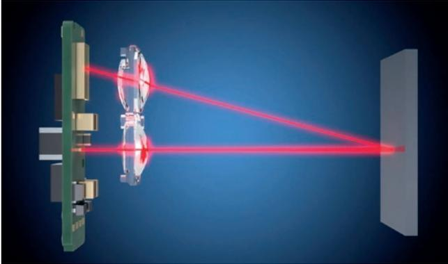
The background suppression feature is based on a distance measurement that involves the calculation of an angle, which is referred to technically as triangulation.
