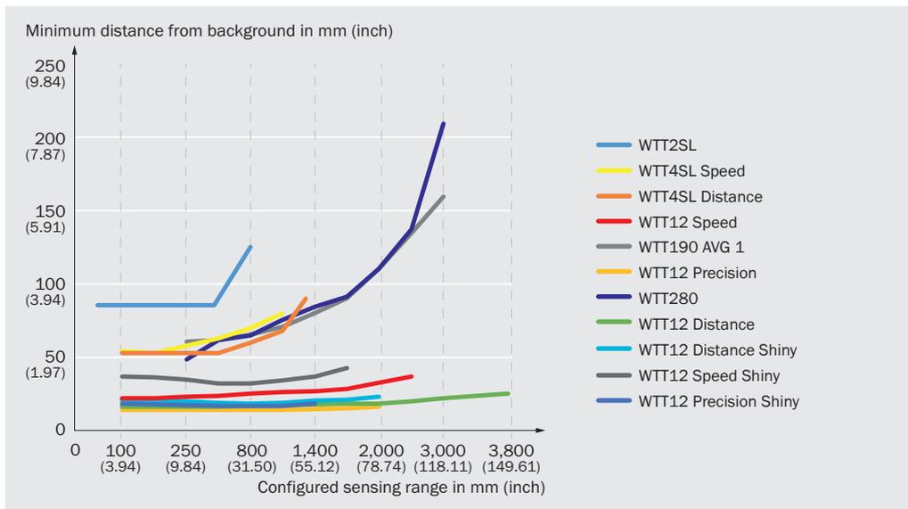
Time-of-flight photoelectric proximity sensors
