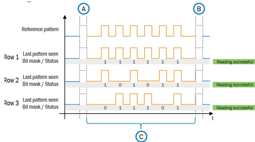
Figure 17: Workpiece carrier and the associated signal schema with pattern clipping: Two signal edges each at the beginning and end of the pattern are cut off and are not included in signal evaluation
