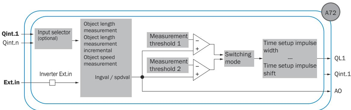
Figure 7: Logical principle of operation A72
