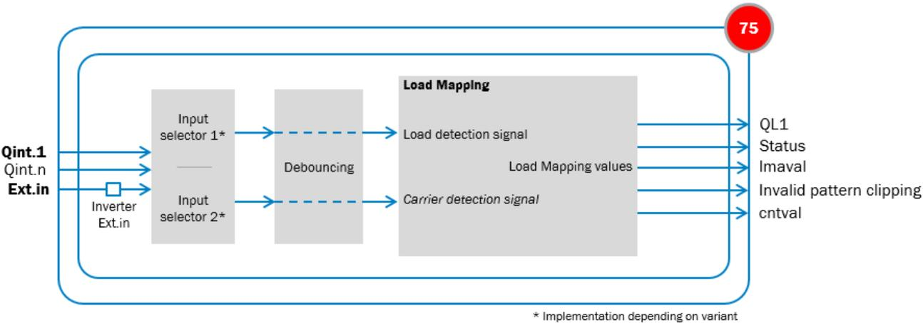
Figure 11: Logical principle of operation A75
