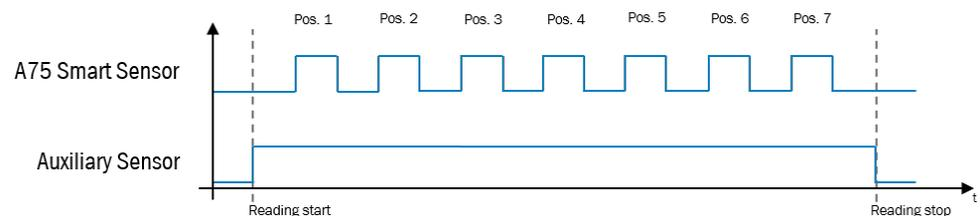
Figure 18: Signal position of A75 Smart Sensor to auxiliary sensor (**Direct object detection, midpoint/width mode**)
