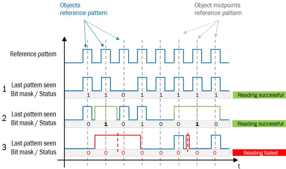
Figure 15: Midpoint evaluation (Direct object detection) signal schema
