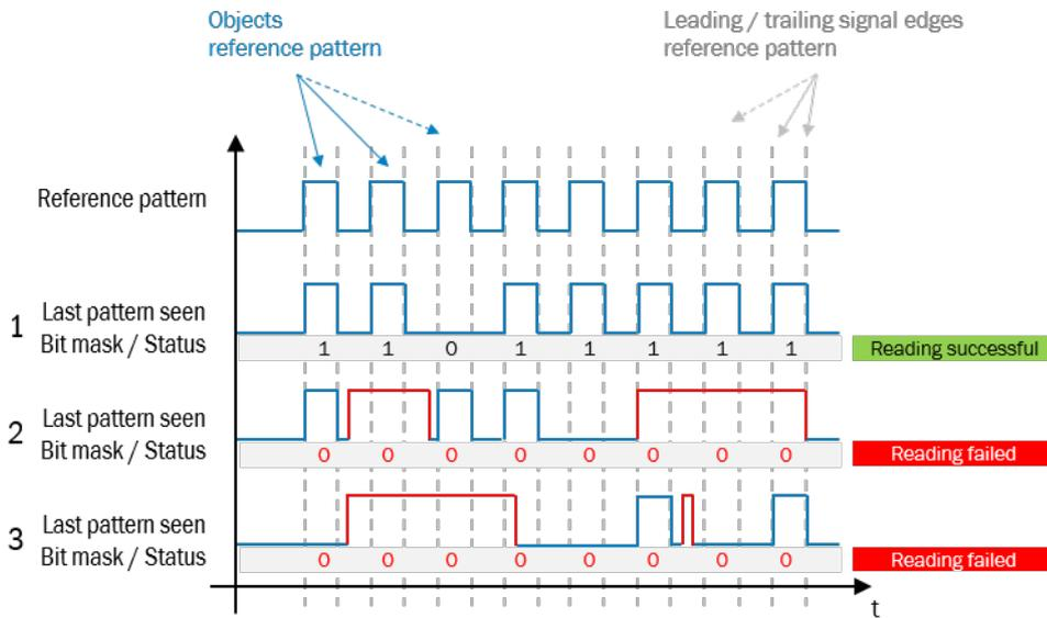
Figure 16: Width evaluation (direct object detection) signal schema
