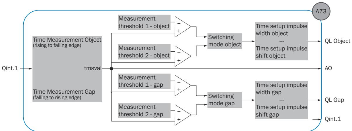
Figure 10: Logical principle of operation A73
