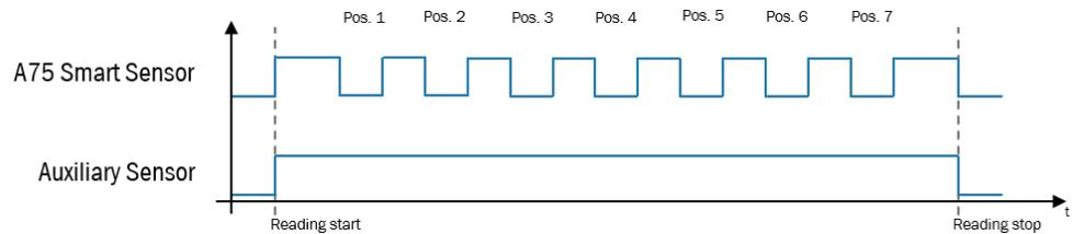
Figure 19: Signal position of A75 Smart Sensor to auxiliary sensor (*Inverse object detection, width mode*)
