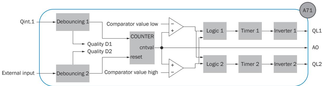
Figure 6: Logical principle of operation A71
