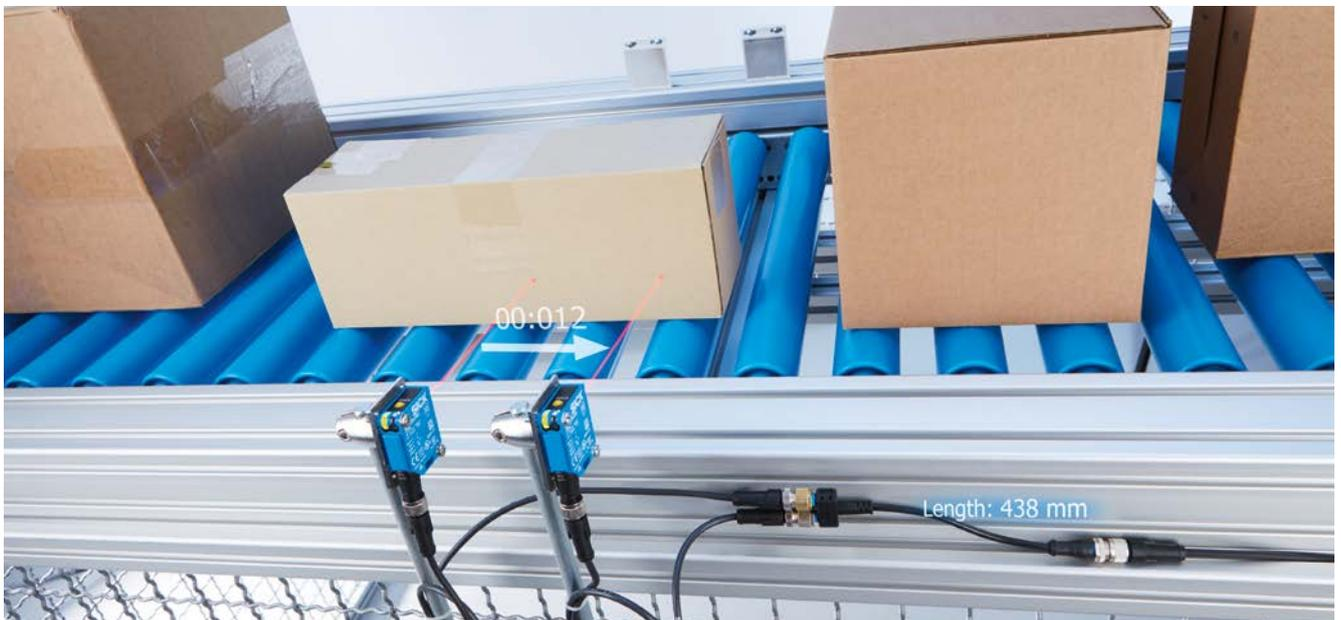
**Examples of Smart Tasks: added value for your application****Speed and length measurement**
