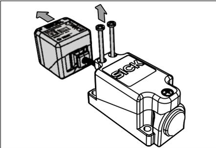
2.2 Swivel or rotate sensor head
