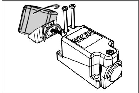
2.3 Push the sensor head back to the base and fasten screws
