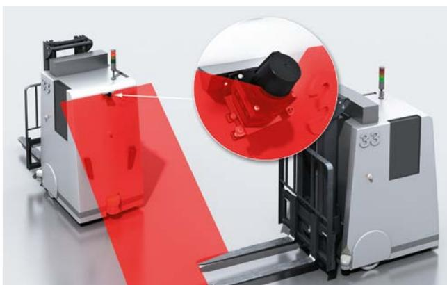
Two-dimensional collision avoidance for automatically guided vehicle systems.
