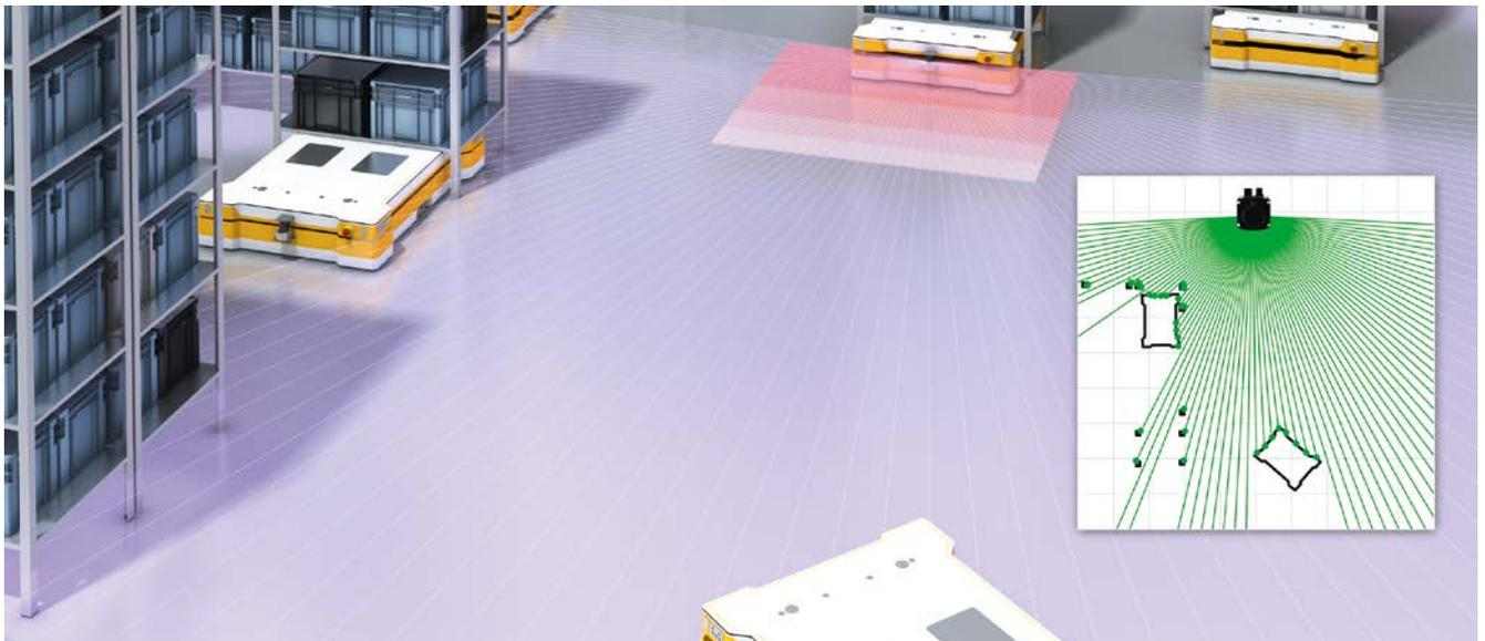
Localization and collision avoidance in automated warehouses.
