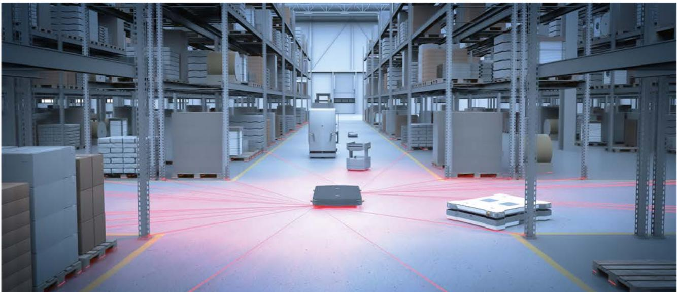
Simultaneous localization and mapping (SLAM).
