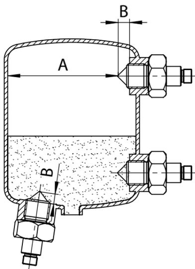
Installation in a pipe for dry running protection.
