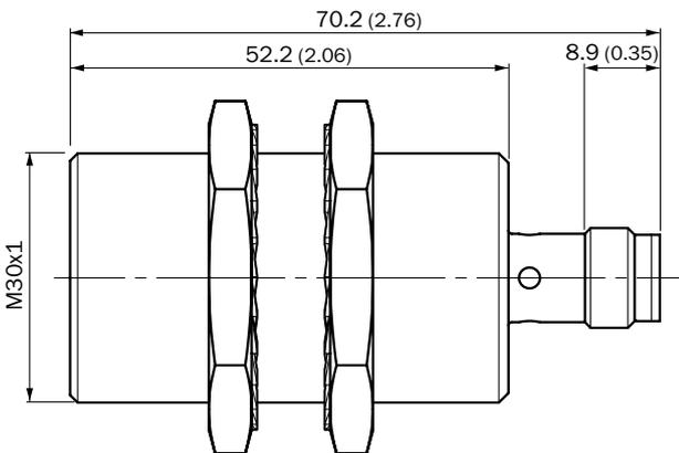
IMC30 Standard, connector M12, non-flush
