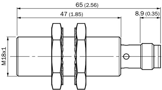
IMC18 Standard, connector M12, non-flush
