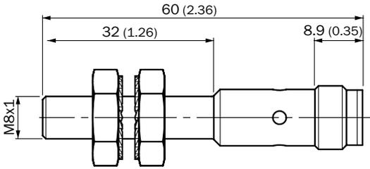
IMC08 Standard, connector M12, non-flush
