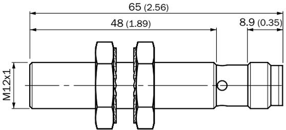
IMC12 Standard, connector M12, non-flush
